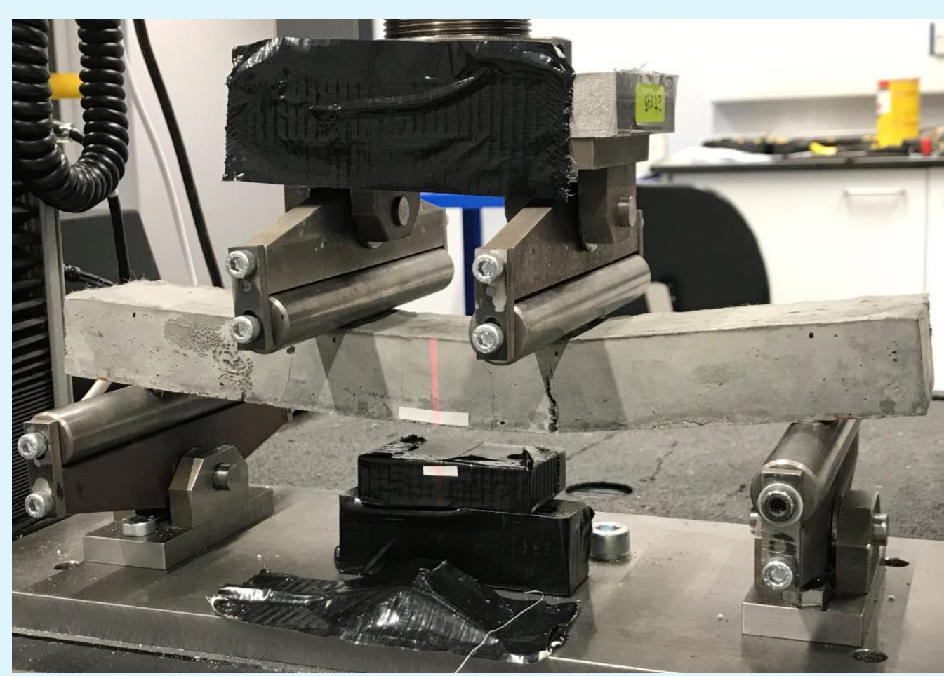
Fig. 3 The setup for four-point flexural tests and large deformation achieved by SHCC
