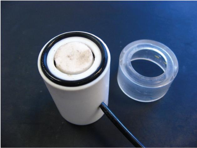
Fig. 10. Faecal pellet crusher developed to measure undrained shear strength of faecal pellets
