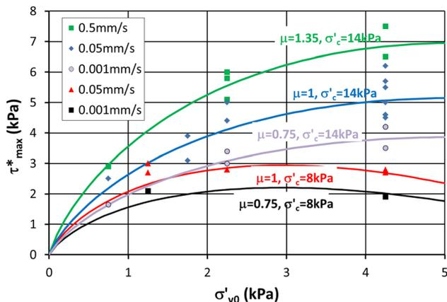
**FIG. 8** Cam-shear data of remoulded, reconstituted West African clay plotted on normalised axes of shear strength and vertical effective stress.
