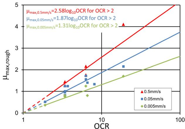
**FIG. 14** Peak apparent friction coefficient  $\mu_{max}$  sliding on a smooth interface, versus initial OCR plotted on semi-log axes.
