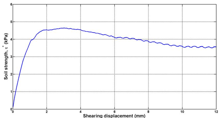
**FIG. 6** Summary of shear displacement to attain soil peak strength.
