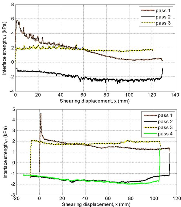
**FIG. 11** Influence of interface roughness on shearing distance required to reach 50 % of  $\tau_{max}$ .
