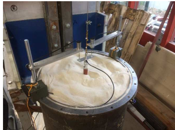
(b) LVDT, Load cell and Pile set-up
