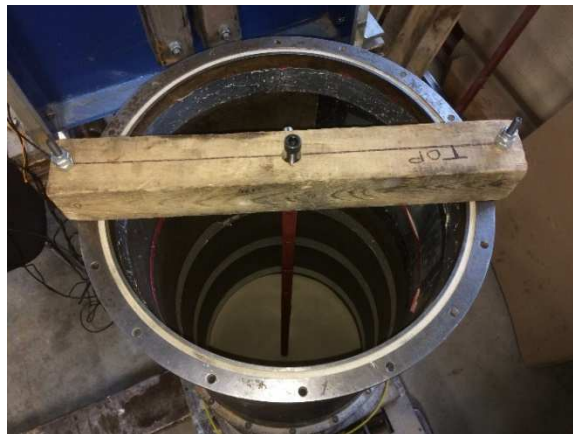
Figure 3.6: Jig holding the pile, whilst sand is poured around it
