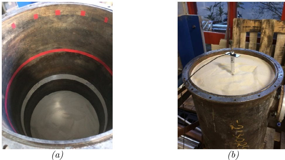
Figure 3.3: Sand container, (a) interior with depth markings, (b) filled with sand
