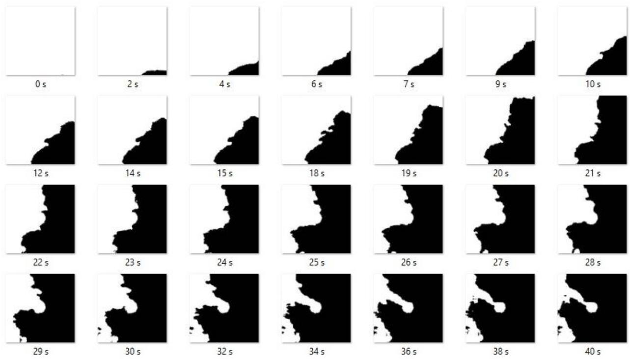
Figure 8.7. "Enveloping" of reinforcement in Experiment 3
