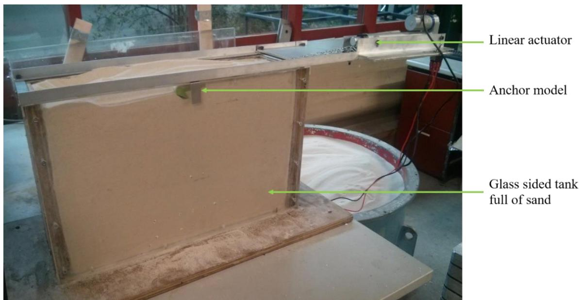
*Figure 20: Preliminary test setup*
