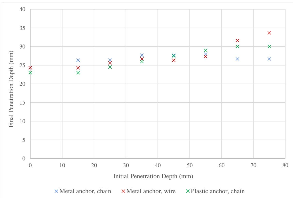
Figure 22: Graph of Halls anchor final penetration depth with varying initial depth in dry sand at 1g, no trendlines have been drawn as there is no clear trend to the data
