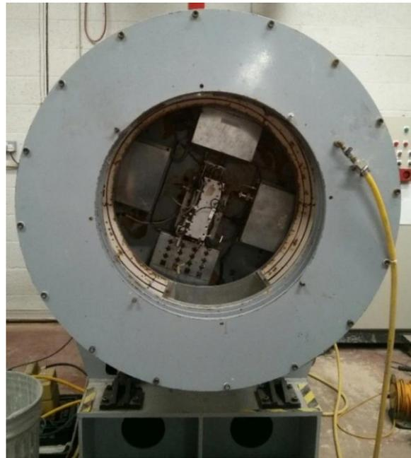
Figure 11: Minidrum centrifuge
