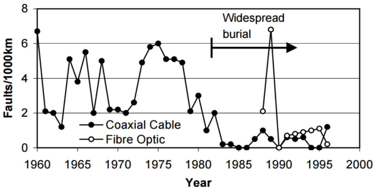
Figure 5: Graph of cable fault occurrence since the introduction of cable burial [13]
