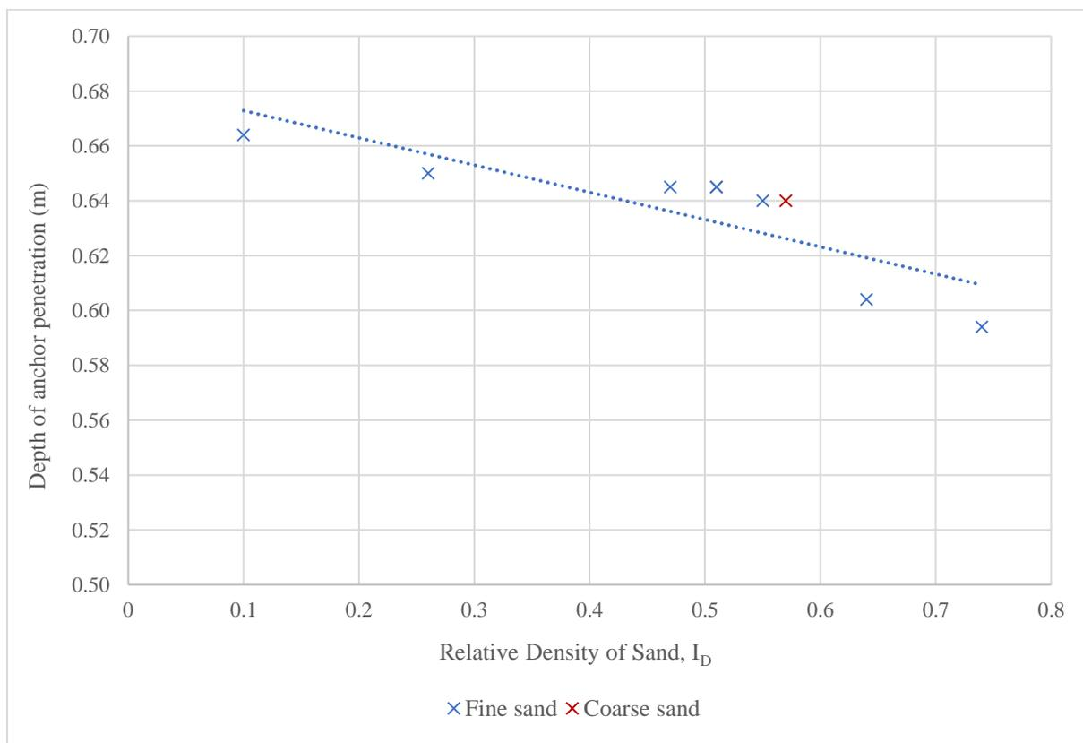
Figure 28: Graph of final anchor penetration depth with varying sand density
