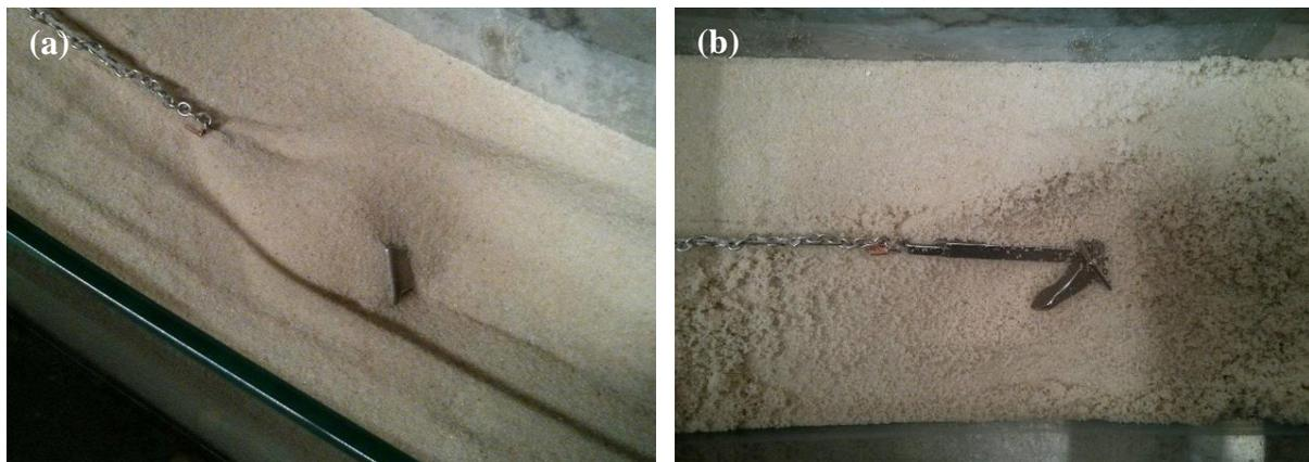
Figure 27: (a) After testing, one side of fluke seen to have twisted out of the sand
