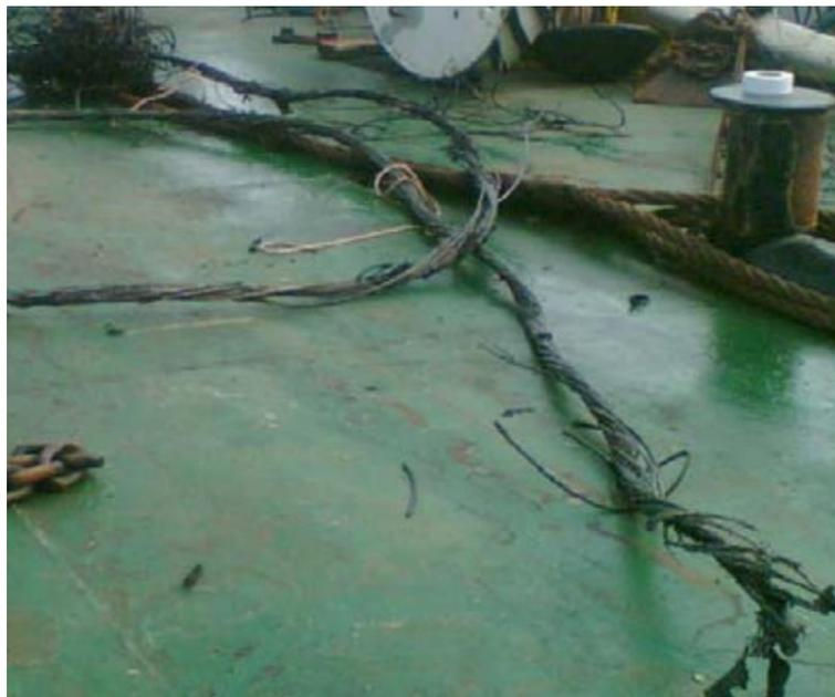
*Figure 2: Cable damage caused by an anchor [3]*
