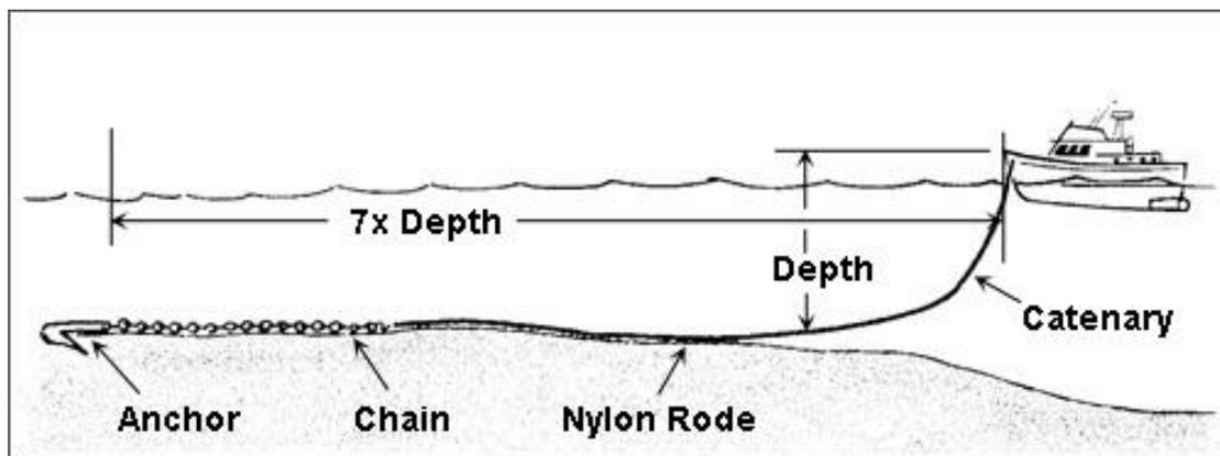
Figure 4: Diagram showing a deployed anchor [10]
