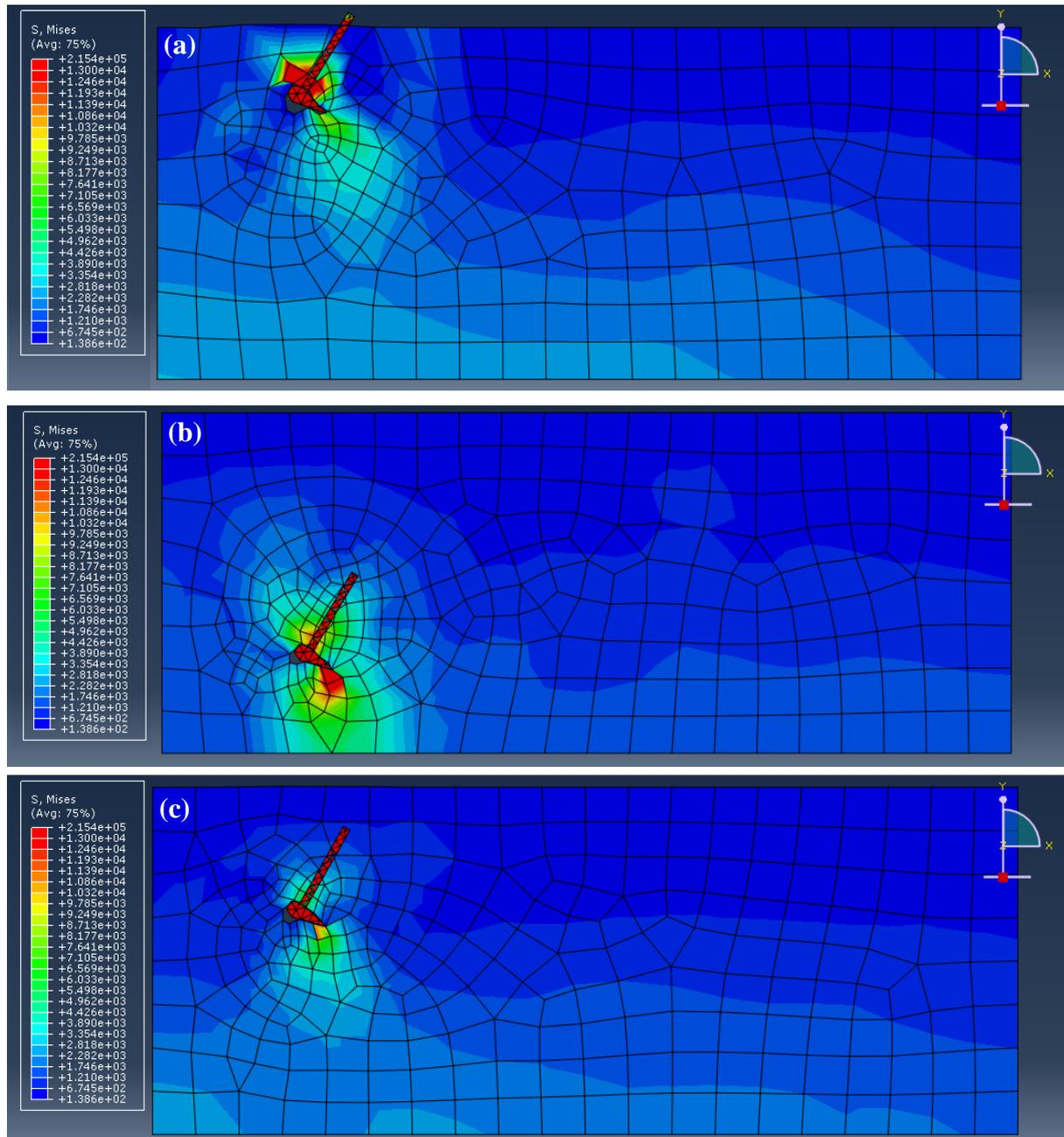
Figure 23: FEA simulation showing the stresses in the sand around the Halls anchor when (a) anchor is buried deep in the sand (b) anchor is near the surface of the sand (c) anchor is close to equilibrium
