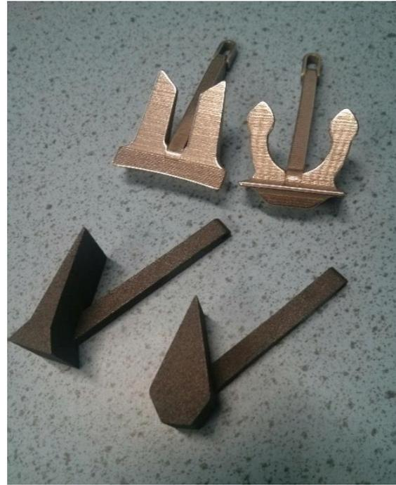
Figure 19: 3D-printed stainless-steel anchor models
