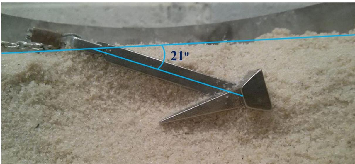
Figure 24: Final orientation of AC-14 anchor after centrifuge Test 1
