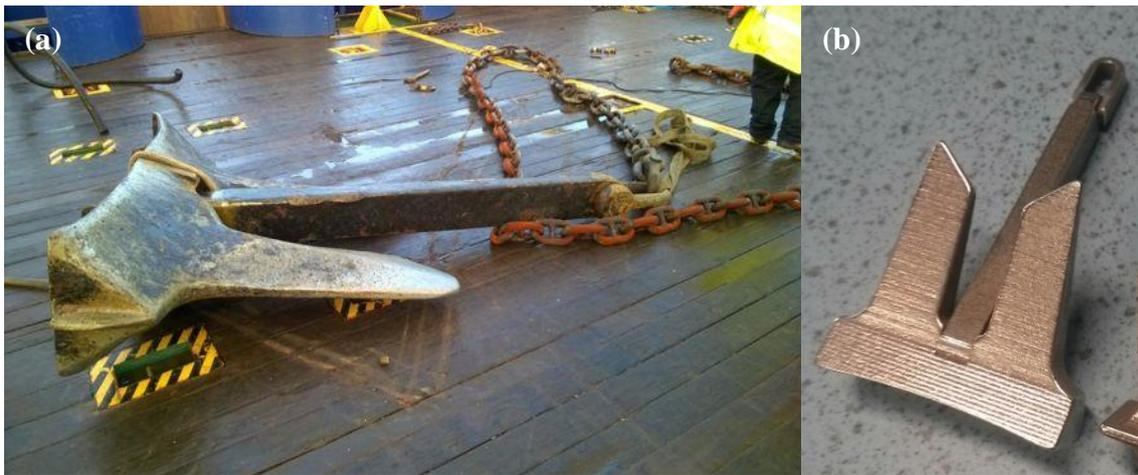
Figure 14: (a) AC-14 anchor that damaged Jersey's cables in November 2016 [19]
