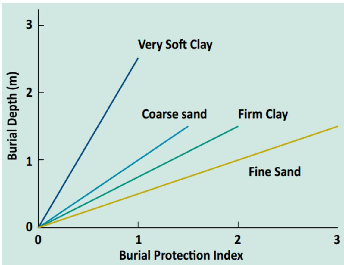
Figure 7: Cable and Wireless Marine guideline for cable burial depth [4]
