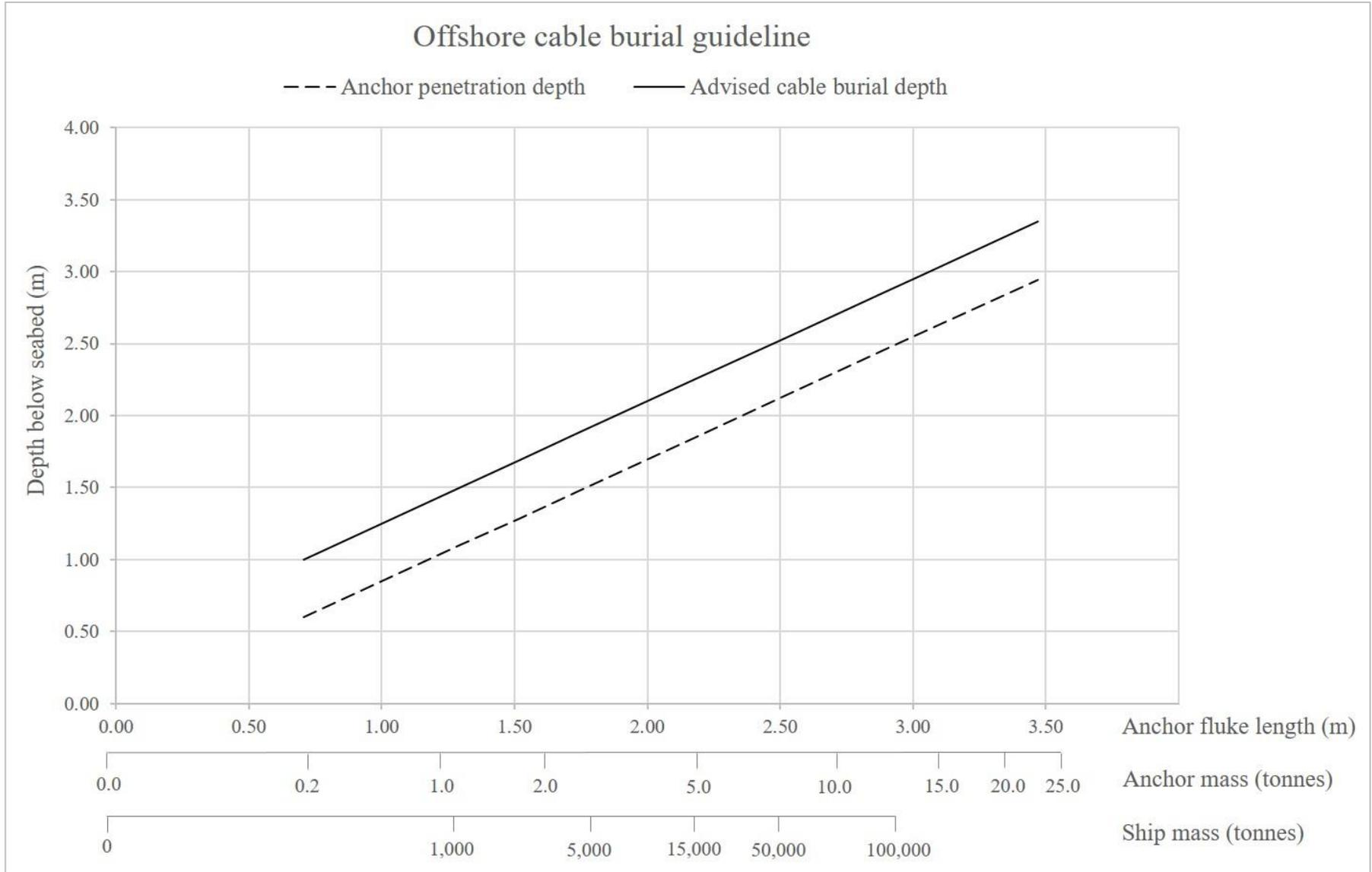
Figure 33: Final guideline for cable burial depth
