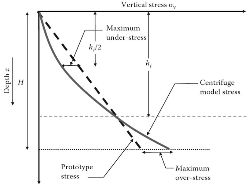
Figure 12: Graph of stress variation in centrifuge model [21]
