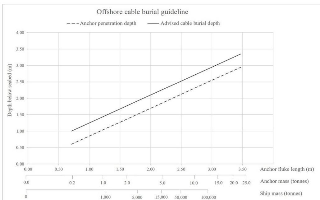
Figure i: New guideline for burial depths of offshore cables
