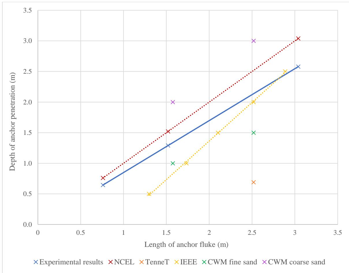
Figure 26: Graph of anchor penetration depth with varying AC-14 anchor size, from various sources
