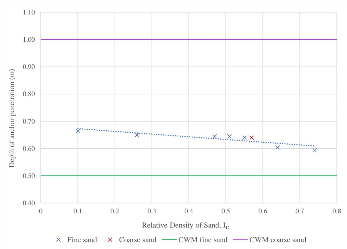
Figure 30: Graph of experimental results and CWM guidelines for fine and coarse sand
