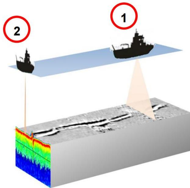
Figure 8: Combined SSS and SES approach to tracking anchor penetration depths [15]
