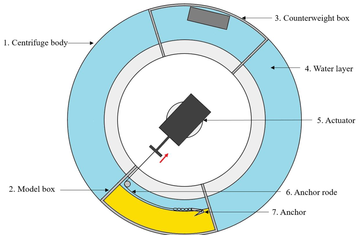
Figure 15: Plan view of the experimental setup
