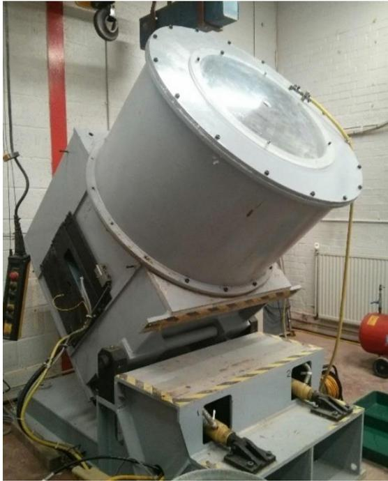
Figure 18: Centrifuge being tilted to the horizontal position for testing
