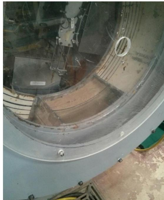
*Figure 17: Model box secured in place in the centrifuge drum*
