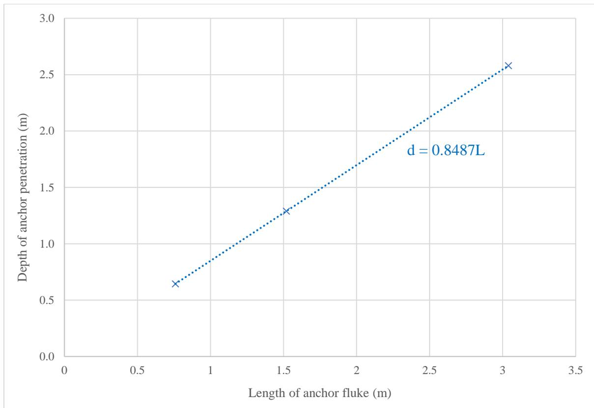
Figure 25: Graph of final anchor penetration depth with varying AC-14 anchor size
