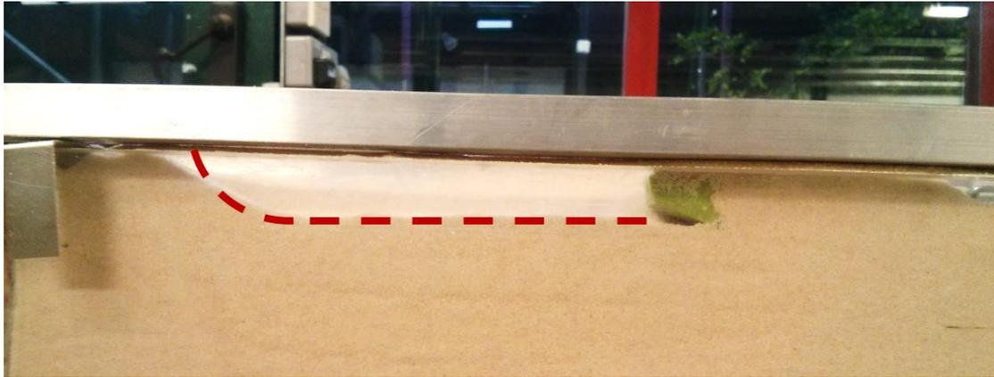
Figure 21: Sand profile after Halls plane strain anchor dragged through sand
