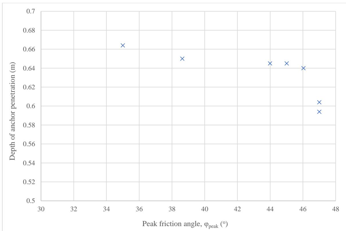
Figure 29: Graph of final anchor penetration depth with varying peak friction angle of sand
