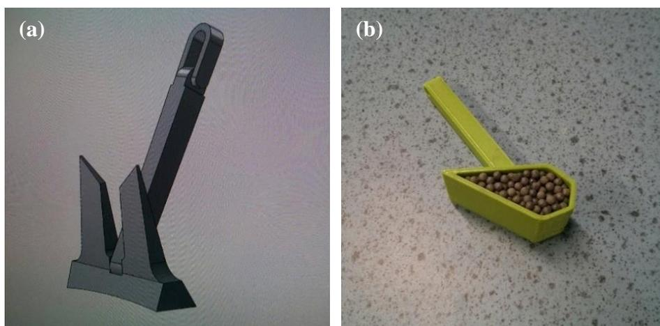
Figure 13: (a) AC-14 anchor modelled in SolidWorks (b) Plastic plane strain Halls anchor filled with lead shot
