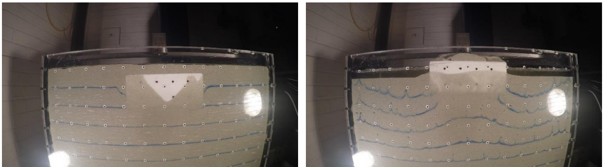
Figure 16 - Test 1 Before and After Shaking
