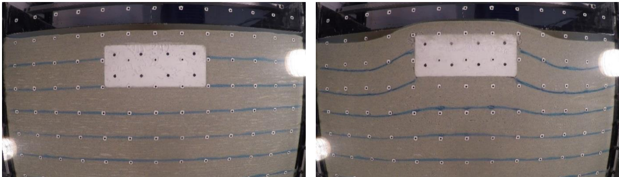
Figure 26 - Test 3 Before and After Shaking
