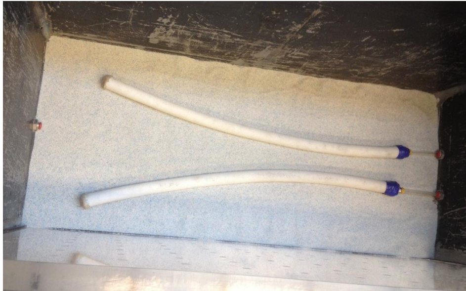
Figure 12 - Porous Saturation Tubes
