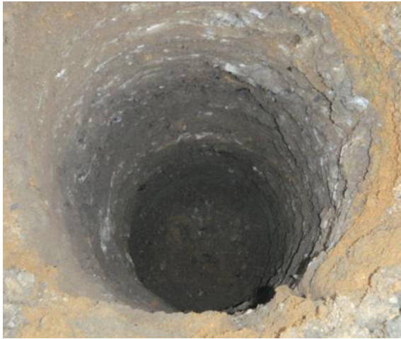
(a) Pre-augered pilot hole — prepared before testing
