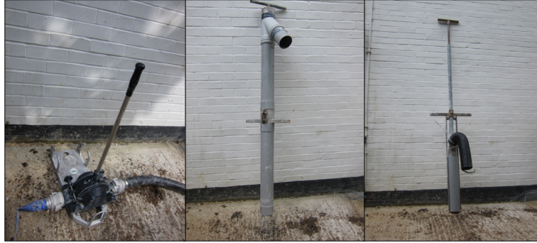
Figure 2: Left to right - The Oxfam diaphragm pump, the Gulper 1 and the Gulper 2
