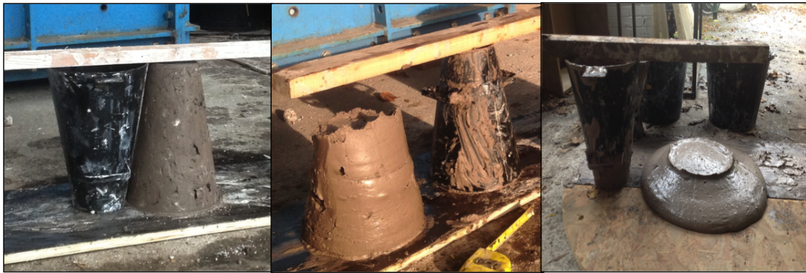
Figure 4: Slump testing: Simulant at 68000Pa, 1300Pa and 300Pa
