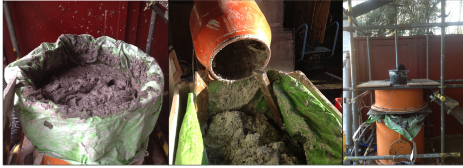
Figure 6: The mixed simulant in the tank, mixing the simulant for testing, testing the Gulper 2 .
