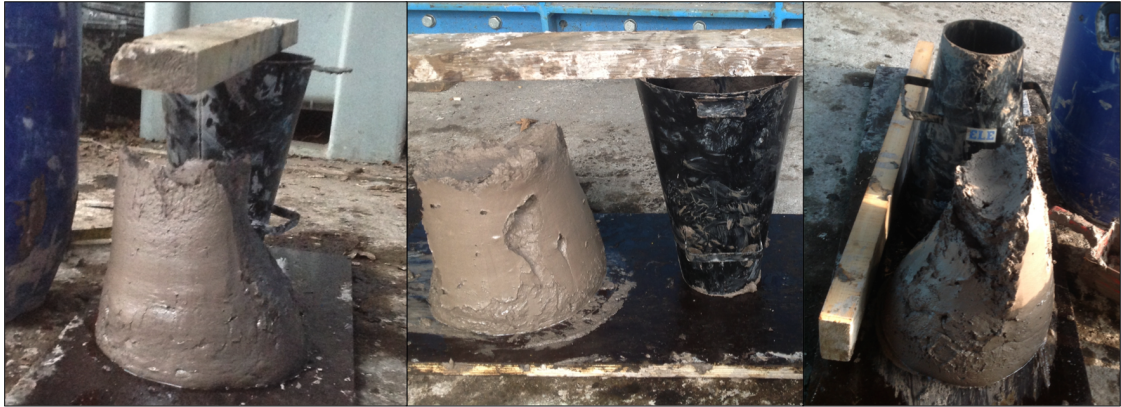
Figure 5: Failed slump tests showing, from left to right: a) the cone being pulled to one side due to the stickiness of the sludge on release, b) voiding due to poor compaction and c) both problems simultaneously
