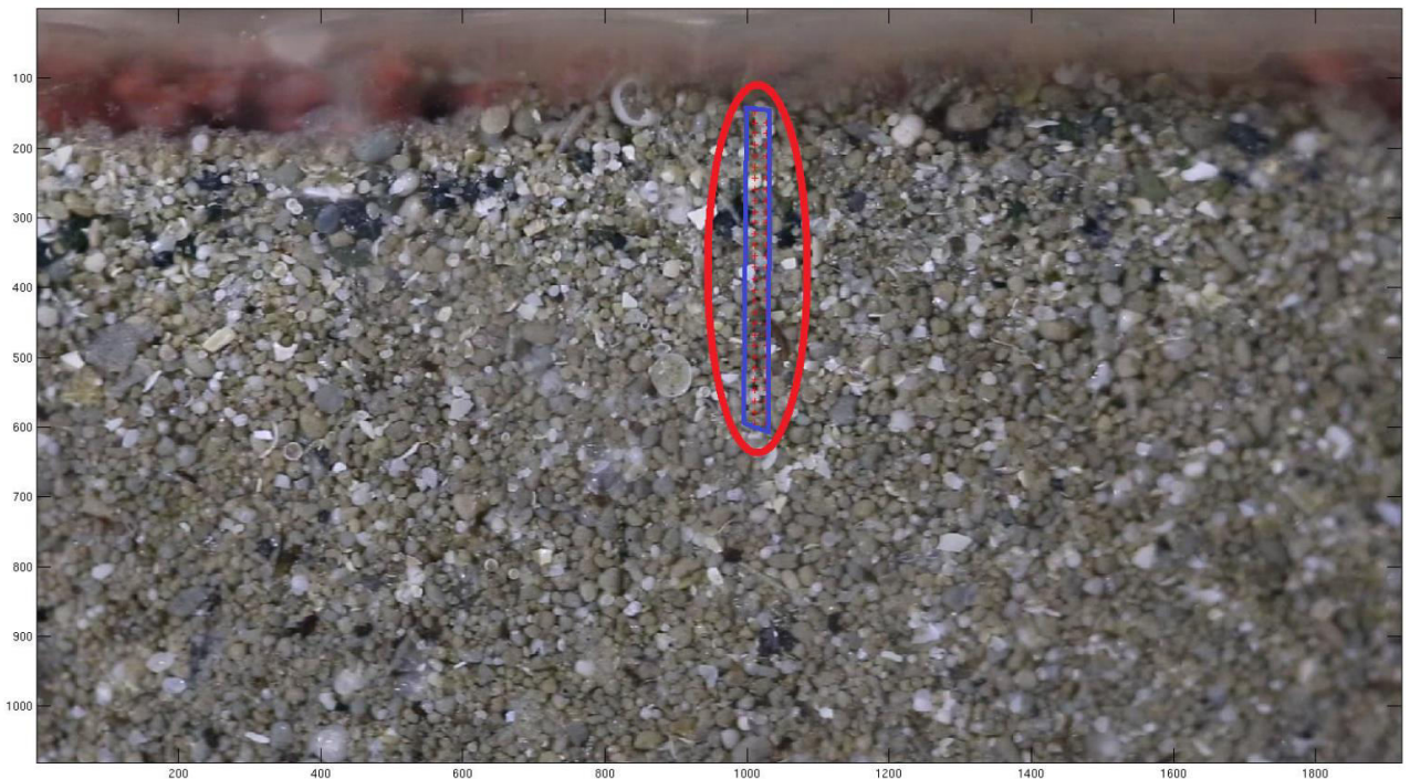
Figure 20 – Mesh used in first PIV analysis (indicated by blue lines)
