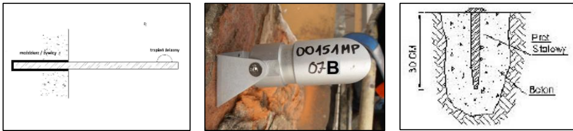
Figure 5.1 Installation of levelling pin, mini prism and ground pin
