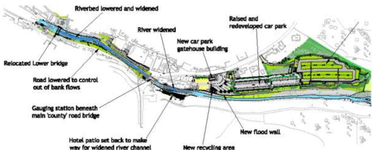
Figure 22 - Implemented flood risk improvement works in Boscastle post-2004 flood 2 .
