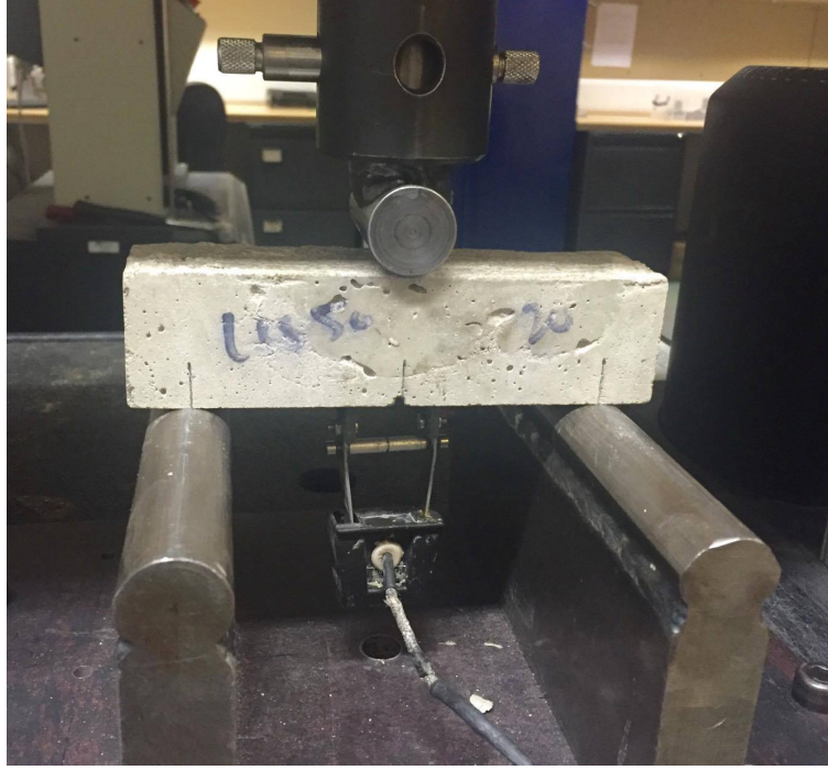
Figure 13: Set up of three-point bending test on Instron ® with strain gauge attached on bottom face
