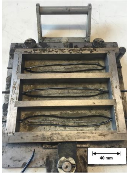
Figure 11: Half cast mould with black speaker cable as formwork for multi-tube network (grey reinforcement bar, discussed in Section 3.2, is also visible)
