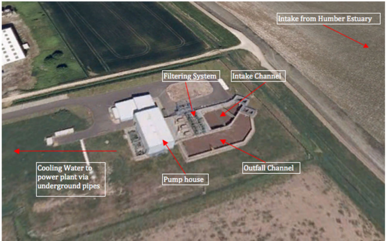
Figure 1.1: Intake System arrangement of SHBPS.
