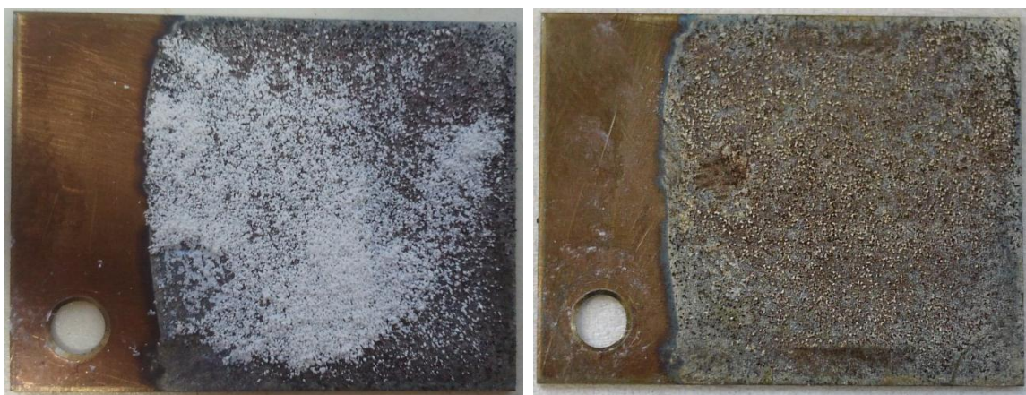
Figure 16: Stainless steel plates using silver paint method – before (left) and after (right) testing in MTBE solution
