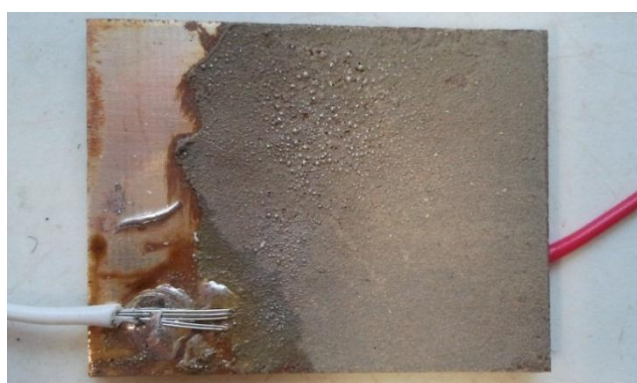
Figure 16: Stainless steel plates using silver paint method – before (left) and after (right) testing in MTBE solution
