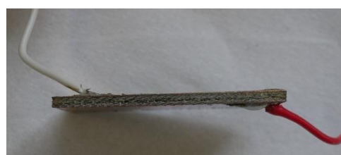
Figure 17: Unprinted circuit board using zinc glue method 1
