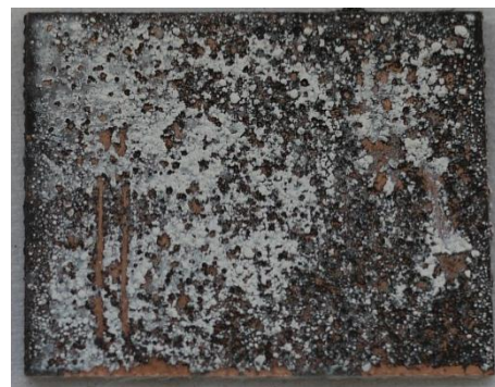
Figure 21 (right): Unprinted circuit board using nickel spray method
