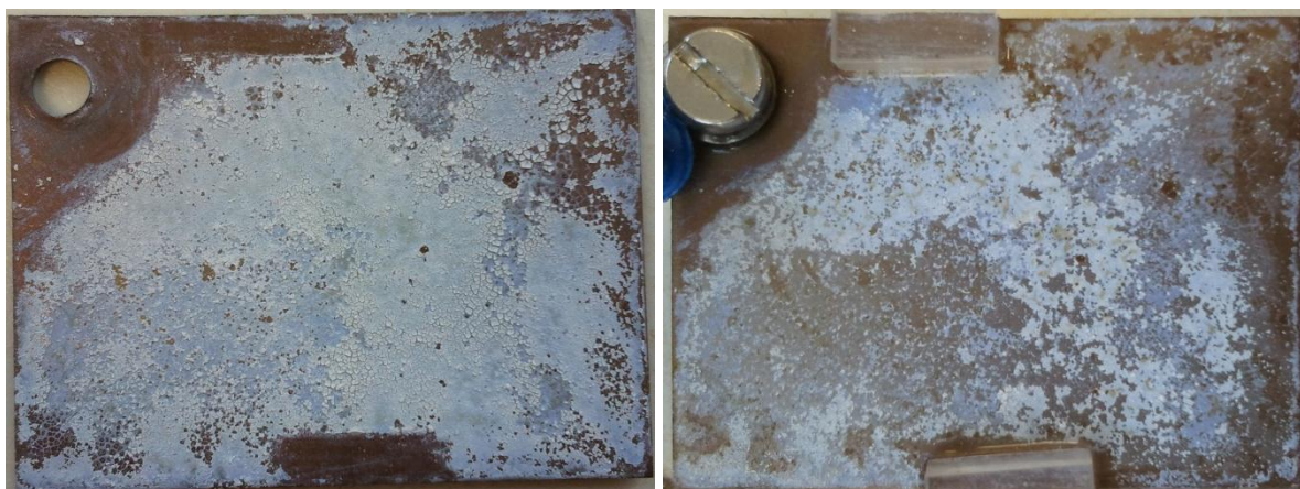
Figure 31: Photos of sensor plate surface taken in January (left) and March (right)
