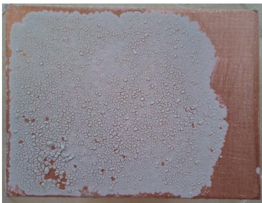
Figure 20: Unprinted circuit board using silver paint & surfactant method – before (left) & after (right) soaking in water for 10 seconds
