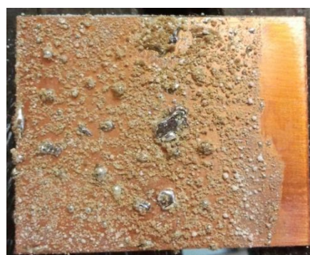
Figure 17: Unprinted circuit board using zinc glue method 1
