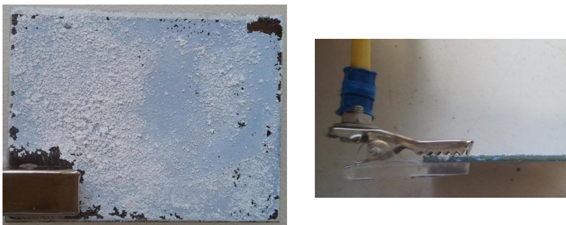
Figure 23: Chromium plated glass using ethanol slurry method and its connection clip
