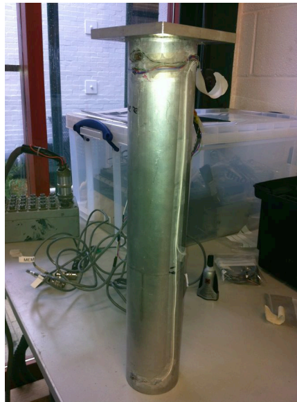
Figure 3.1: Instrumented model monopile.
