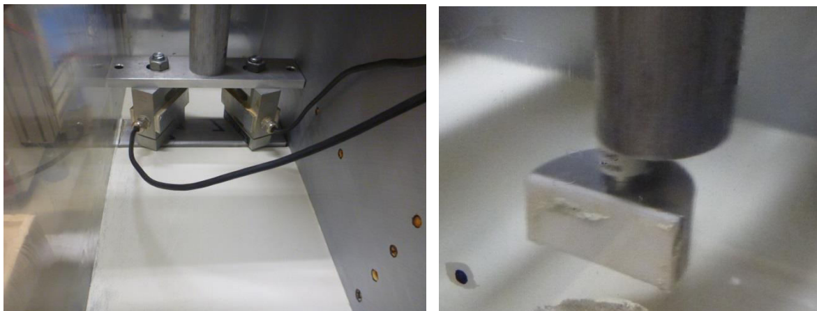
Figure 3-2: Final designs of Strip Footing (left) and Semi-Circular Footing (right) used in experiments
