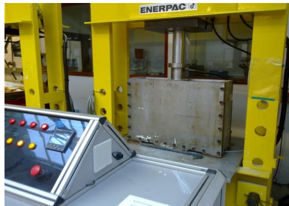
Figure 3-1: Automatic Consolidometer and testing tank used
