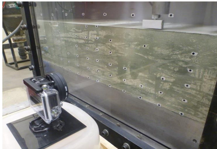
Figure 3-6: Illustration of 'texturing' used on clay
