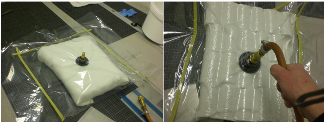
Figure 9.2.3.3 (above left), 9.2.3.4 (above right) and 9.2.3.5 (below). Sealing the samples, applying vacuum and placing in kiln
