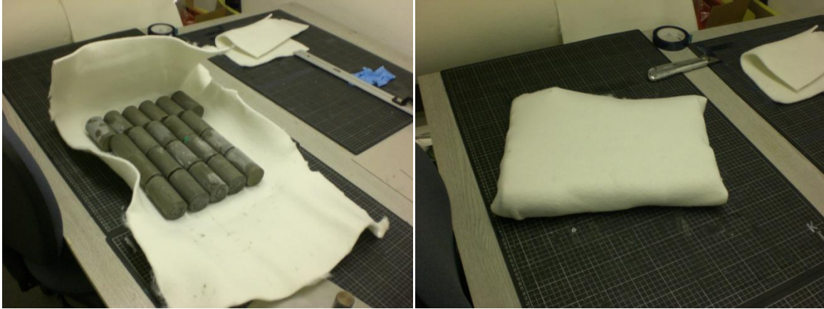
Figures 9.2.3.1 and 9.2.3.2 – Wrapping the cement samples in breather blanket
