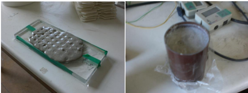
Figure 9.1.3 (left): Leaving small samples to set – thick residue on top can be scraped off. Figure 9.1.4 (right): A large sample setting
