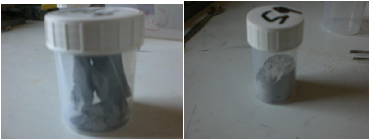
Figures 9.3.1 (left) – Collecting fragments of sample for SEM analysis (N.B. these would be fragmented further until a few mm in size). Figure 9.3.2 (right) Sample in powder form for XRD analysis.
