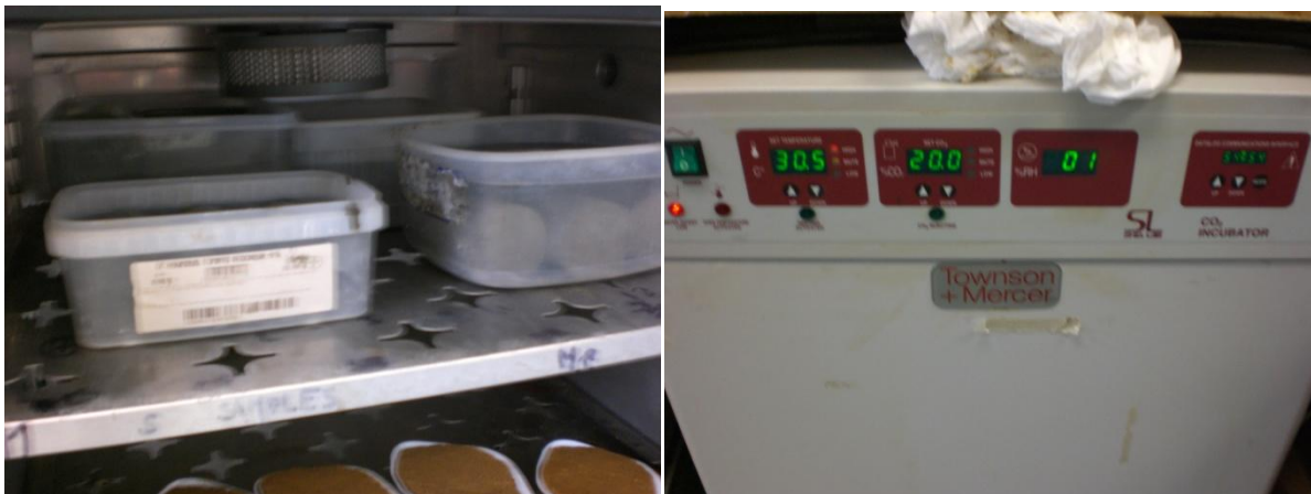
Figures 9.2.4.1 (left) and 9.2.4.2 (right) - Placing submerged samples in incubator and setting the temperature and CO 2 concentration.
