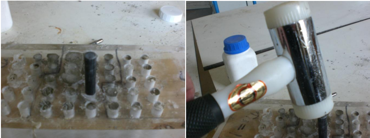
Figure 9.2.5.2 (left) and 9.2.5.3 (right). A hammer and nylon rod are used to force the samples out of the Perspex sheet
