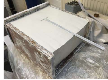
Figure 14: Model pile installation in clay
