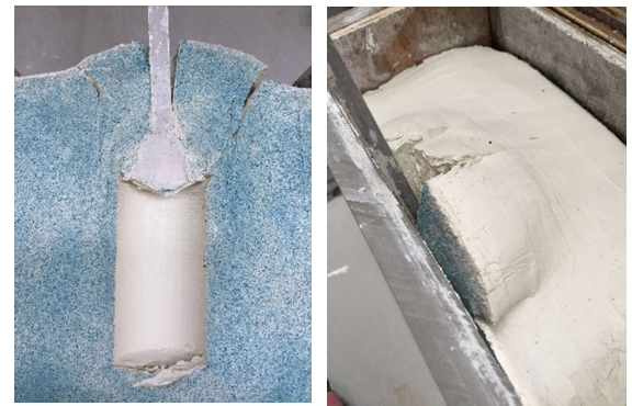
Figure 35: Failure soil wedge with fully developed tension cracks elevation view (left); top view (right)
