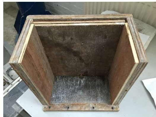
Figure 9: Extra wooden boards fixed to test container (with perspex front face removed)
