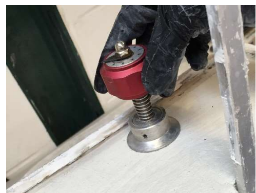
Figure 10: Hand vane shear test to find c_u of clay
