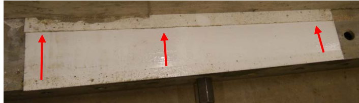
Figure 5.6 The movement of Teflon® sheets after bending test
