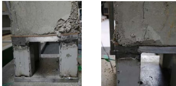
Figure 5.2 Local failure at the corners of the specimen, with the base plate buckled.
