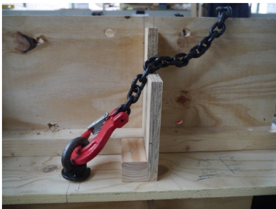
Figure 3.3 Lifting arrangement with specialist lifting rig
