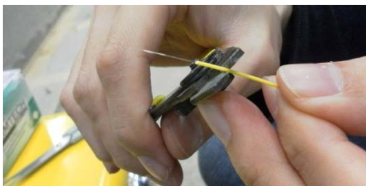
Figure 4.6 Removal of protective layers
