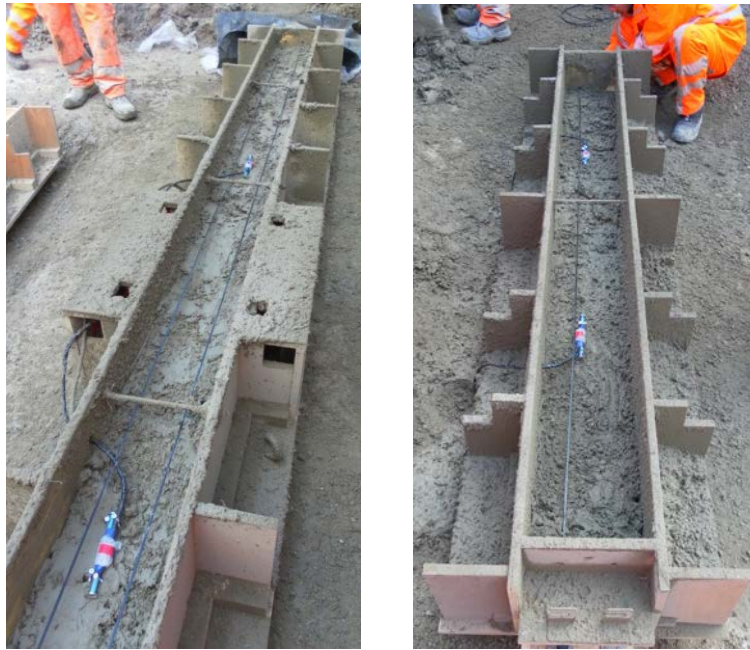
Figure 4.3 The layout of instrumentations (Left: beam, Right: column)
