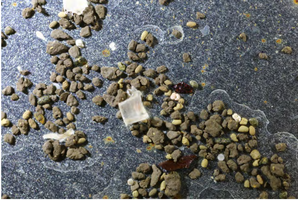
Figure 16: A photo taken after material trapped in sieve larger than 300\mu\text{m} are dried. Pellets photographed here shows two distinct colour. The pale greenish-brown pellets are glauconised and hardened faecal pellets. (Kuo, 2011) The cuboid-like material can be identified as a diatom.
