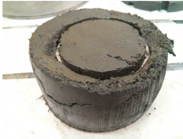
Figure 17: Cutting ring seen to be pushed into a disc of core sample.
