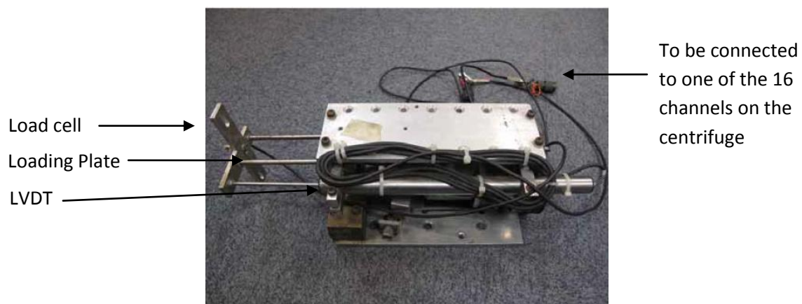
Figure 3-3 Actuator assembly fitted to the minidrum centrifuge (photo: Wang, 2012)
