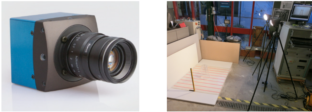
Figure 3.6: High-speed camera (left) and set up (right) used for recording the slump tests
