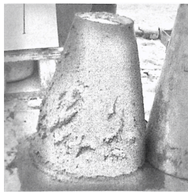
Figure 2.10: Voids and tears produced by tempering of grout in the lower portion (Warner, 2004, p. 149)
