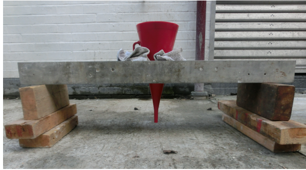
Figure 3.7: Set-up for Marsh funnel flow experiments
