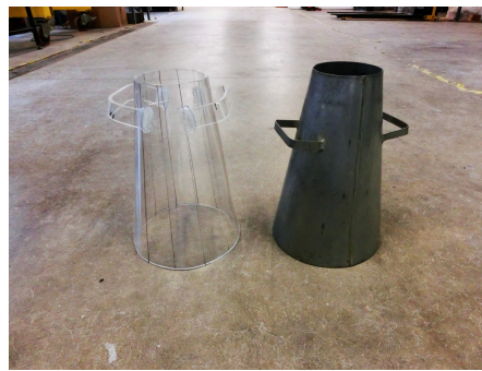
Figure 3.4: Special transparent acrylic slump cone made to allow high-speed camera to record grout flow and a standard metal slump cone
