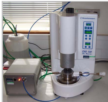
Figure 3.8: Bohlin rheometer used for testing the shear stress and shear rate measurement (Eisa, 2008, p. 76)
