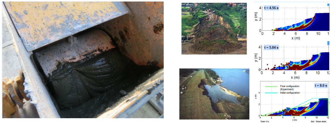
Figure 1.1: Cement-based bentonite grout in mixing process (left) and modelling of large-scale landslides using MPM code (right)
