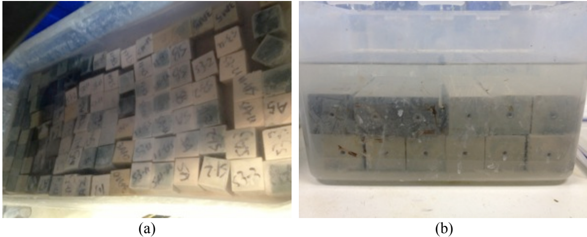
Figure 3-3 The submerged samples, curing in water tank (a) UCS cement cubes (b) submerged shrinkage cement prisms
