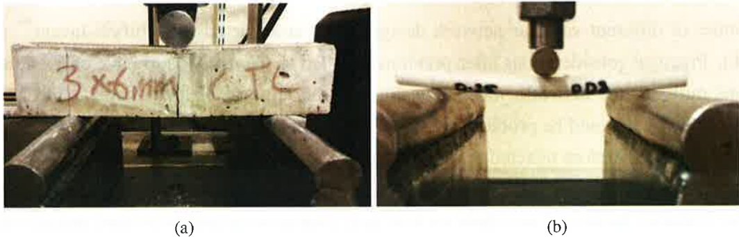
Figure 16: Three-point bending in the Instron ® Universal Testing System. (a) Typical mortar specimen and (b) 3D printed tube, showing support imperfections on the compressive side.
