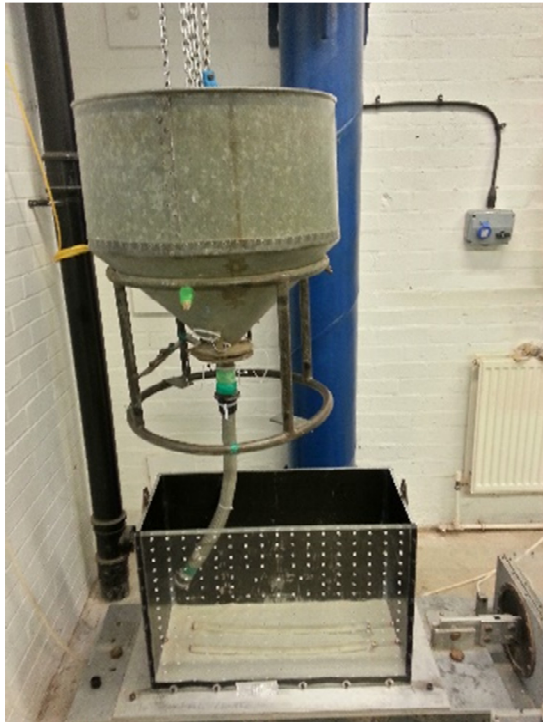
Figure 29 - Sand pouring – sand hopper and test container
