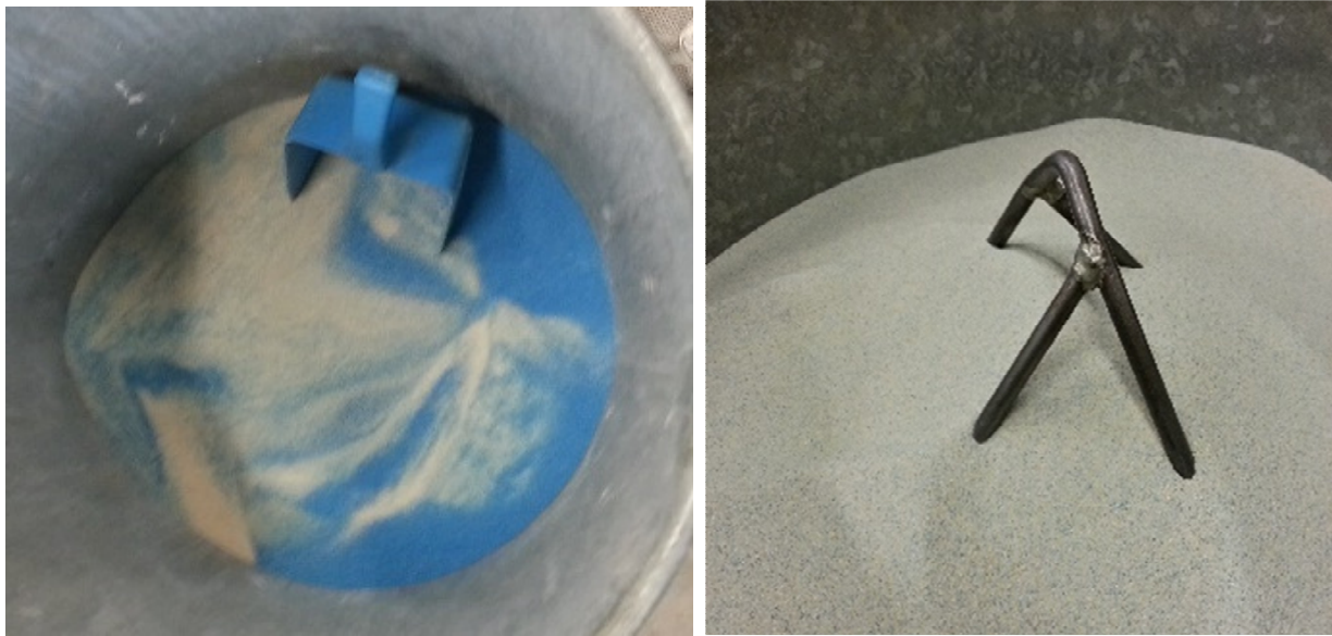
Figure 9 - 10:1 ratio PIV sand mix before and after mixing
