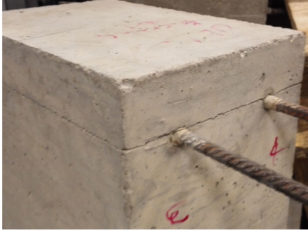
(a) Image of splitting failure across whole length crack
