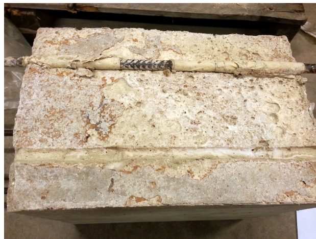
Figure 7.2: Aluminium Crack sample at level of foil crack after testing
