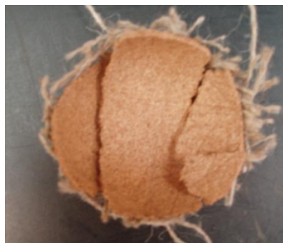
Figure 21 Damage to ball after 80 'overs' of loading
