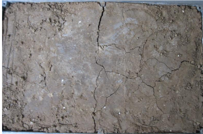
Figure 12 Pitch surface after 30 bounces. Water content – 0.108
