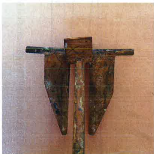
Figure 27: Asymmetric anchor flukes
