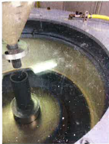
Figure 16: Clay spreader funnel
