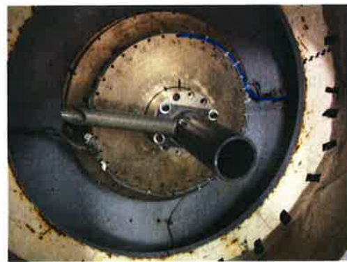
Figure 17: Spreader device mounted in centrifuge
