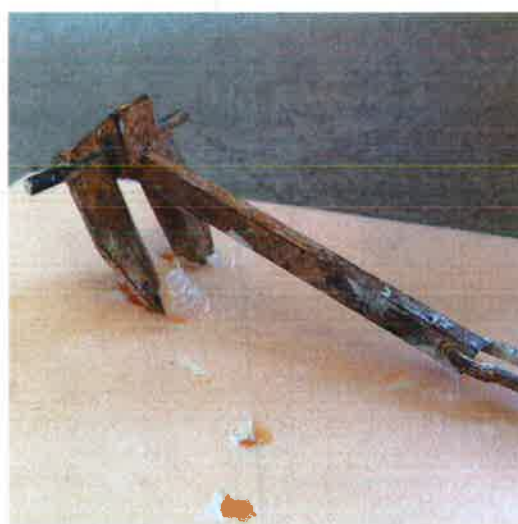
Figure 28: Anchor twisting when pulled
