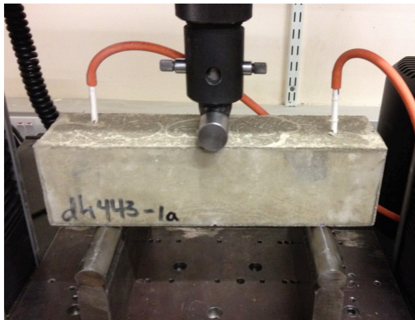
Figure 14: Photograph showing a specimen undergoing three-point bend testing. Orange rubber tubes attached to the white inflow and outflow pipes of the network.
