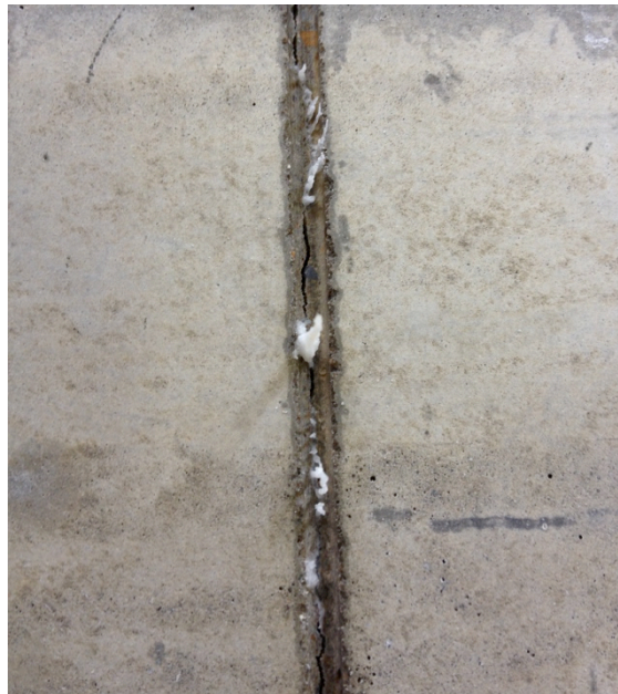
Figure 25: Photograph showing crystals that grew within the cracks of control samples during the healing time within the water bath.
