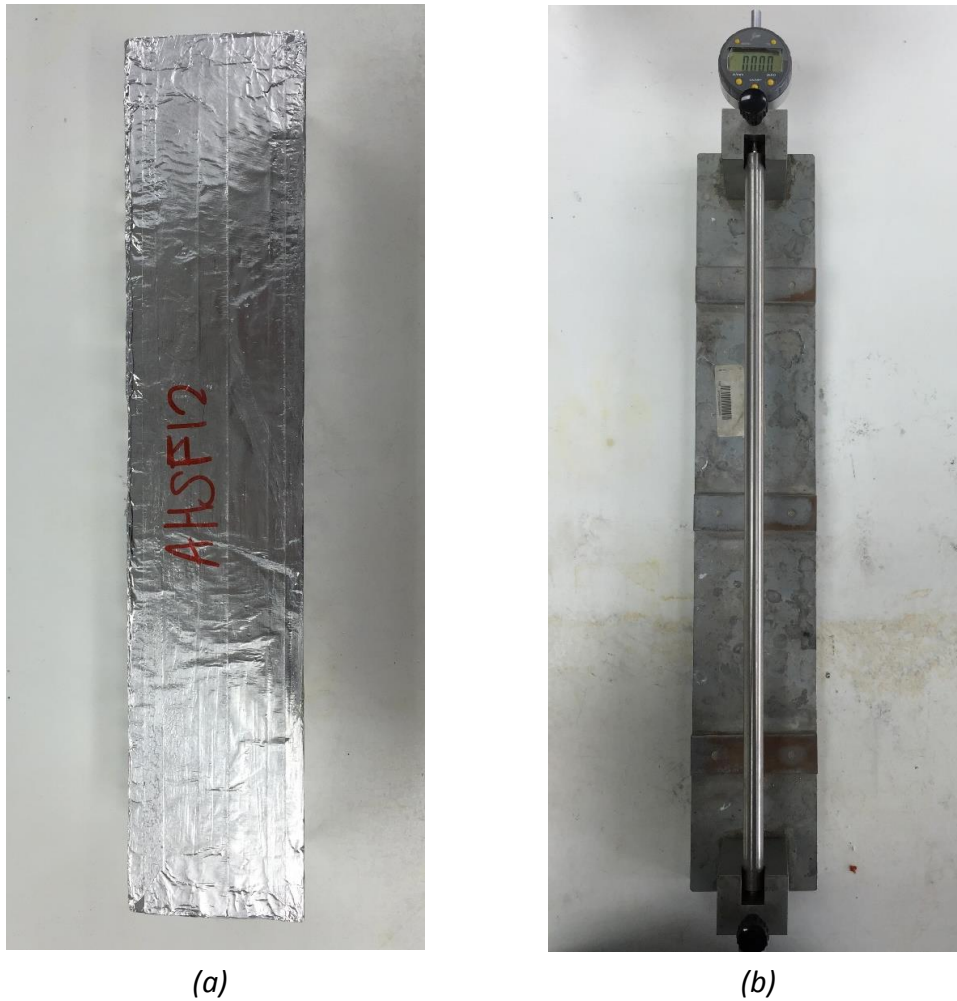
Figure 9: (a) Shrinkage prism; (b) Shrinkage testing apparatus, including reference bar and mechanical displacement gauge
