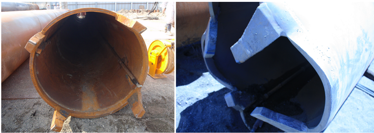
Fig. 2-6: Undeformed (left) and yielded (right) pile base due to the extremely hard ground condition.
