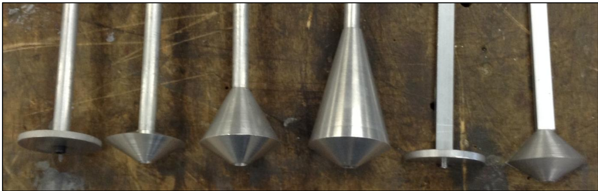
Figure 5: A selection of the model under-reamed piles, with both half space models shown on the far right.
