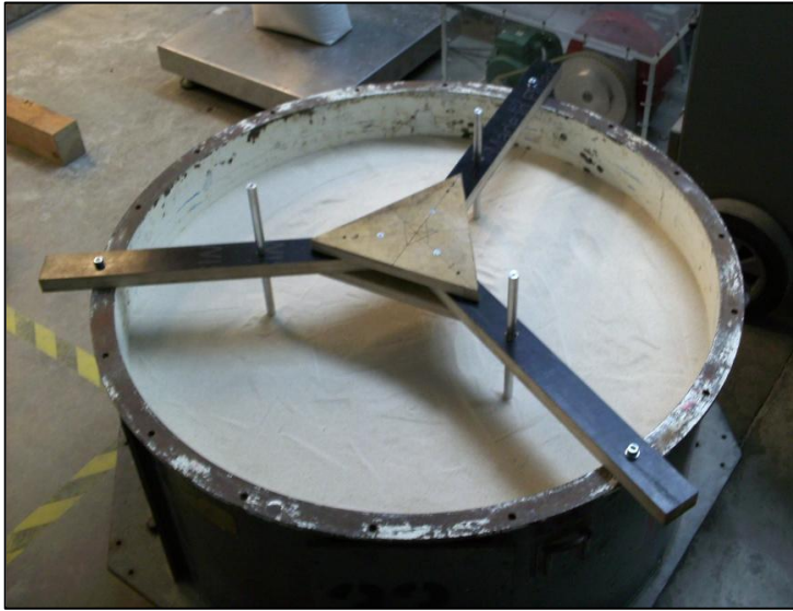
Figure 7: Pullout test jig, securing the piles in place during sand pouring and vibro compaction.
