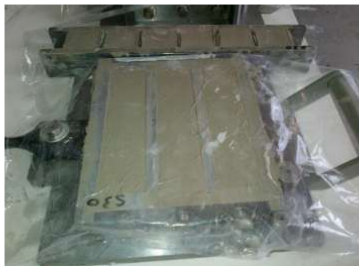
Figure 3.2: Cement paste in moulds undergoing curing
