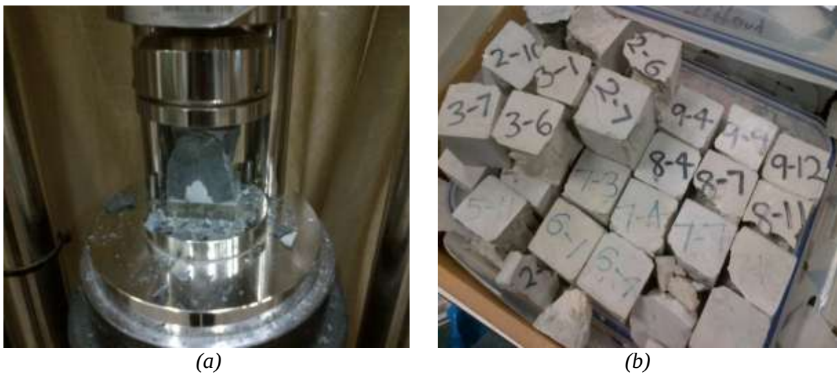
Figure 3.6: (a) Cement paste cube after UCS testing, (b) Collection of UCS tested cubes
