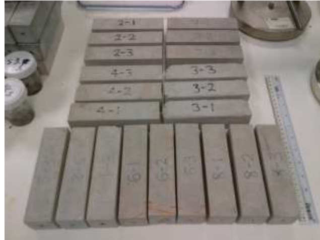
Figure 3.10: Prisms used to observe cement paste shrinkage
