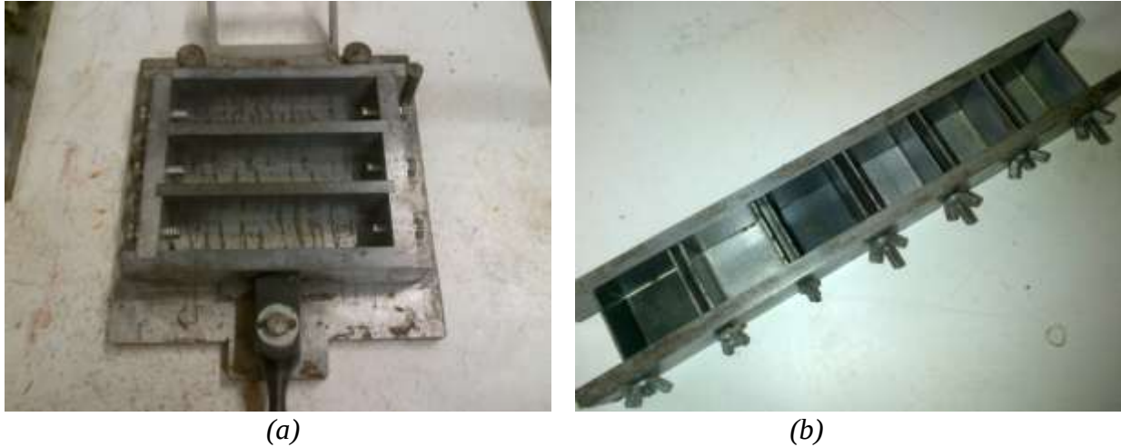
Figure 3.1: (a) Moulds for cement paste prisms, (b) Moulds for cement paste cubes
