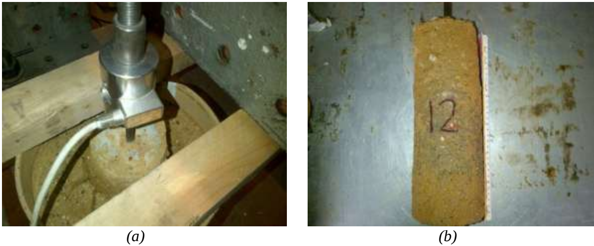
Figure 4.4: (a) Load cell and pile during pull-out test, (b) Removed pile after pull-out test
