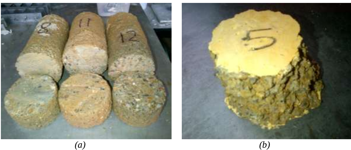
Figure 4.5: (a) UCS samples trimmed from base of piles (b) Sample after UCS testing
