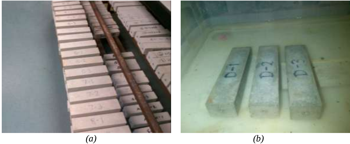
Figure 3.3: (a) Dry curing of prisms on racks in room conditions, (b) Wet curing of prisms submerged in a water tank
