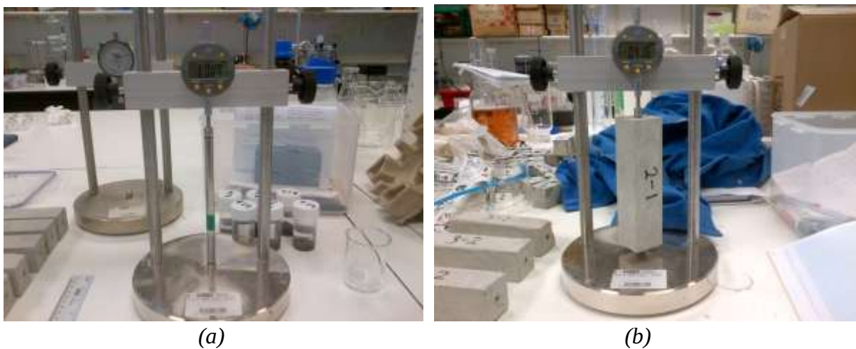
Figure 3.4: (a) Calibration of length comparator with standard rod, (b) Measuring the length of a prism with the digital length comparator
