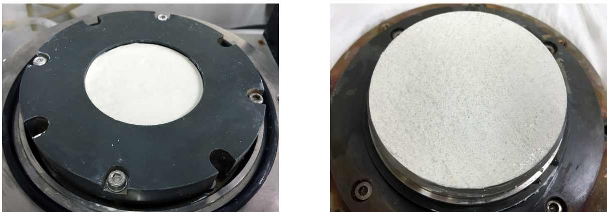
Figure 3.3 - Photographs of soil samples prepared for testing (left) - 100% kaolinite clay (right) - 50% kaolinite clay, 50% Hostun sand by weight
