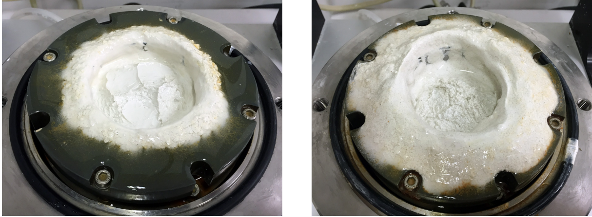
Figure 4.22 - Photographs showing extruded material at the end of tests on a sample made up of 100% kaolinite clay (left) and a sample of 50% kaolinite clay mixed with 50% hostun sand (right)
