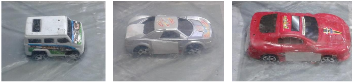
Figure 4 The small, medium and large model vehicles in the water flume. Left: small, Middle: medium, Right: Large
