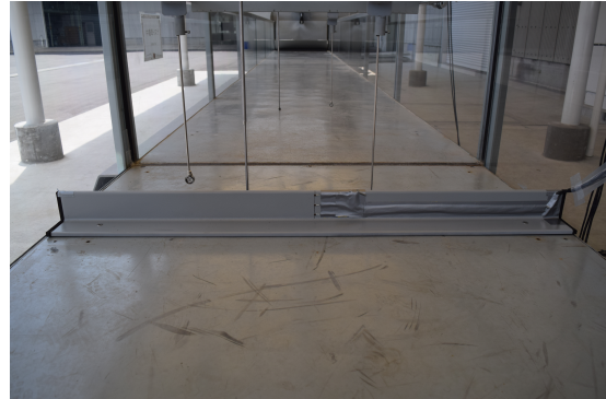
Figure 7: Giken Tsunami Simulator. View from behind the 10 cm model wall. Wave sensors in view
