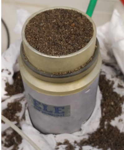
(a) Compacted sample in triaxial cell. Notice thin yellow membrane
