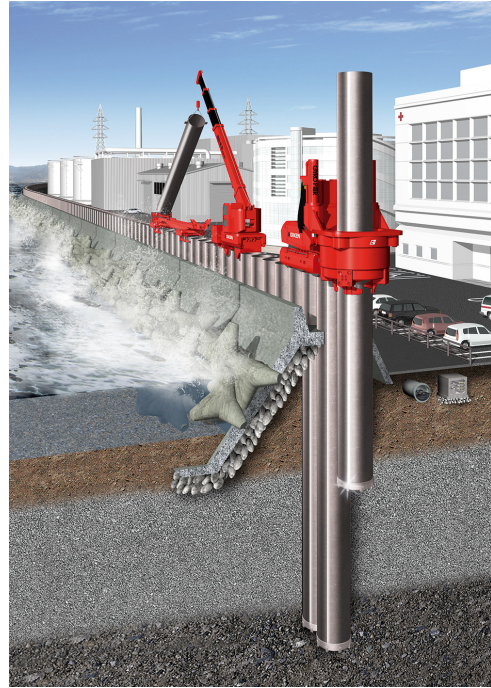
Figure 4: Pile wall jacked in by GRBS
