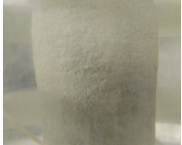
(b) Triaxial sample failure by bulging
