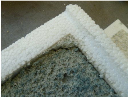
Figure 43: Poor cube corner quality
