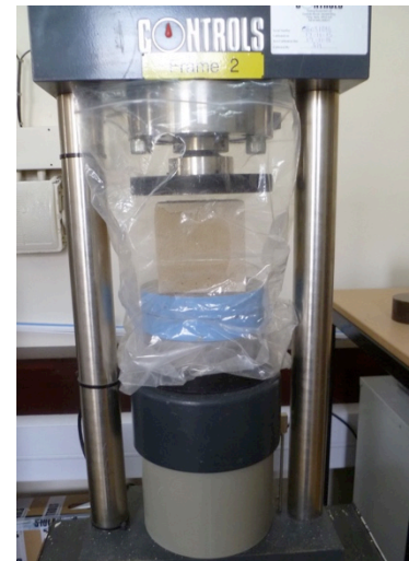
Figure 18: Controls C250kN compression frame
