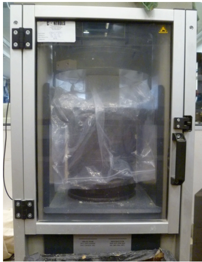
Figure 17: Controls C4600 2000kN compression frame
