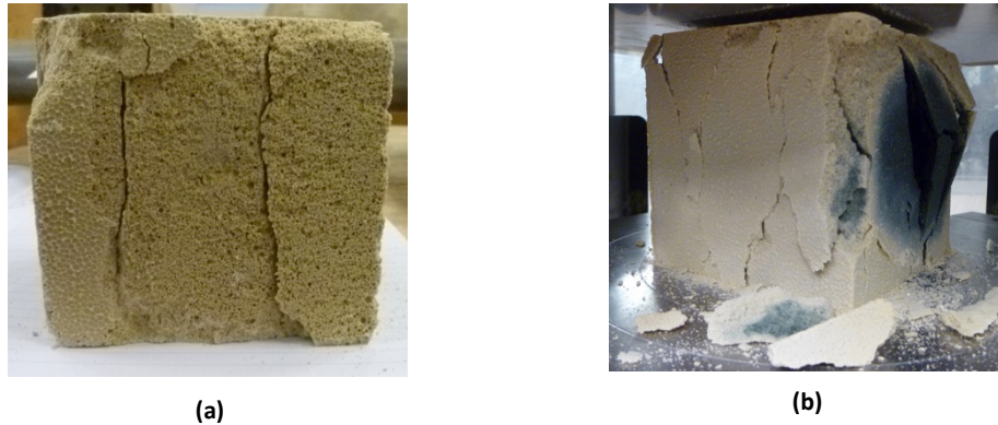
Figure 30: Compression test failure mechanisms
