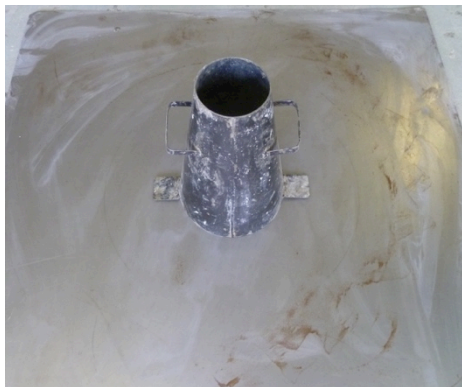
Figure 14: Slump flow test equipment. Note the marked circle for measuring the t_{500} time.
