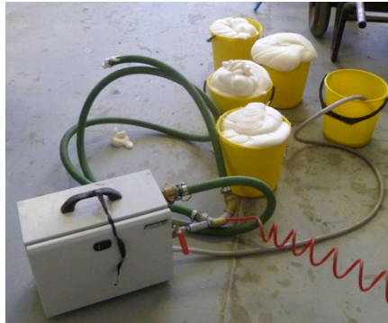
Figure 6: Set up of ProPump Engineering Ltd.'s JFG 200 Foam Generator
