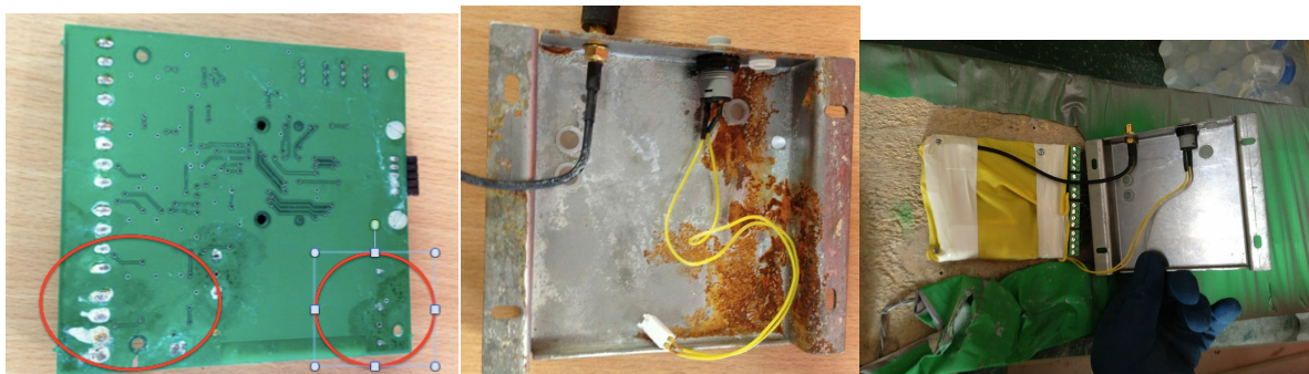
Figure 9.13: (a) Left: Damaged PCB board by oxidation (b) Middle: Damaged Sensor node casing by oxidation (c) Right: Repaired and protected sensor node
