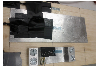
Figure 9.5: Setup for calibration of strain gauges and comparison of attachment method
