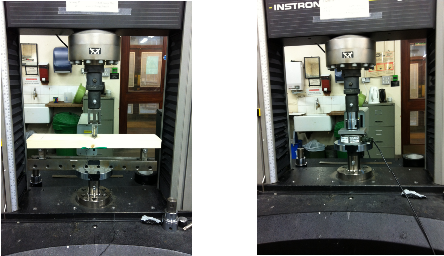
Figure 9.3: Experimental setup for Calibrations of a) Left - Strain gauges (3-point bending test), b) Right - load cells (axial compression)
