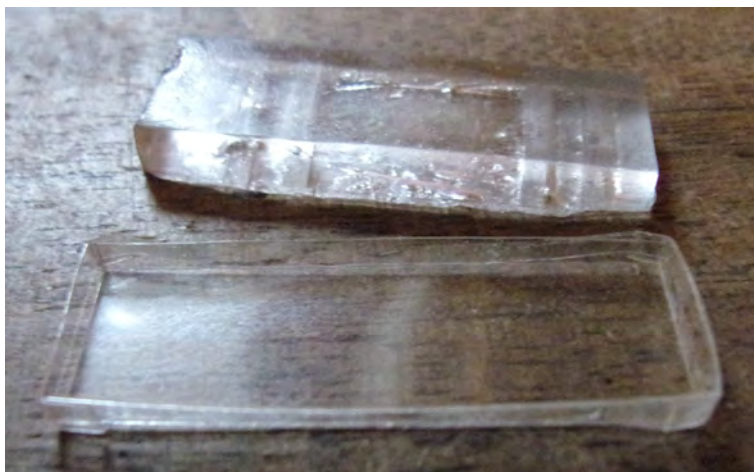
Figure 6: Transparency sheet box used with a top sheet to produce sample. Sample also shown.
