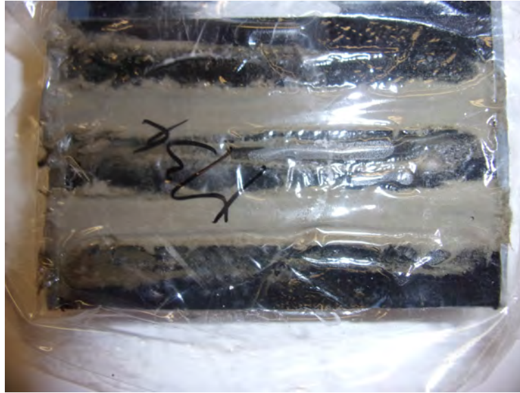
Figure 11: Mould used for casting cement paste prisms. 2 prisms curing.
