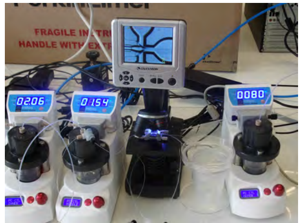
Figure 10: Set-up using 3 pressure pumps.
