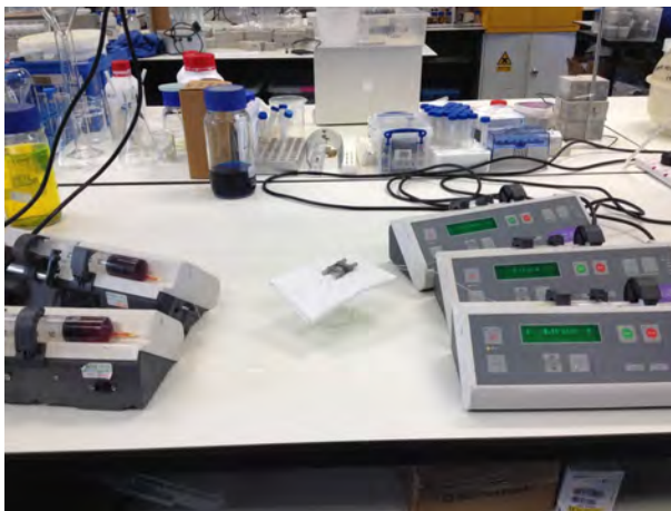
Figure 9: Set-up using syringe pumps.
