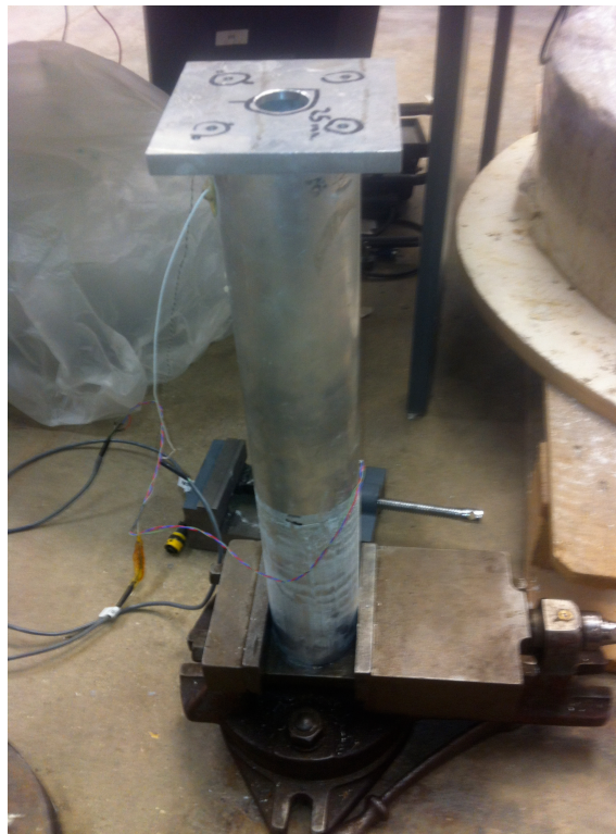
Figure 3.2. Monopile clamped at base for cantilever testing
