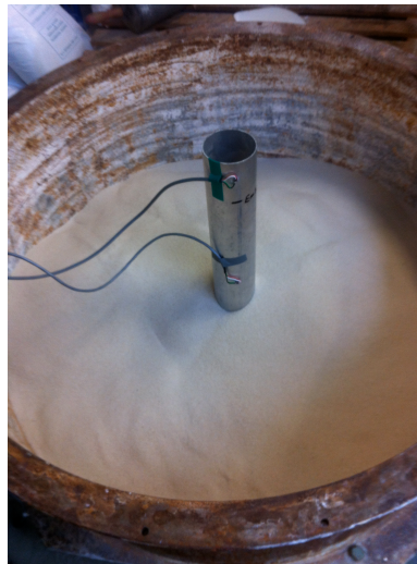
Figure 3.7. Pile installation in process
