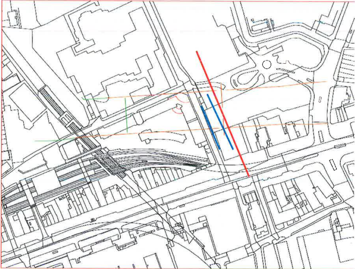
Figure 6. Settlement monitoring arrays (red – greenfield LP, blue – structural BRE)
