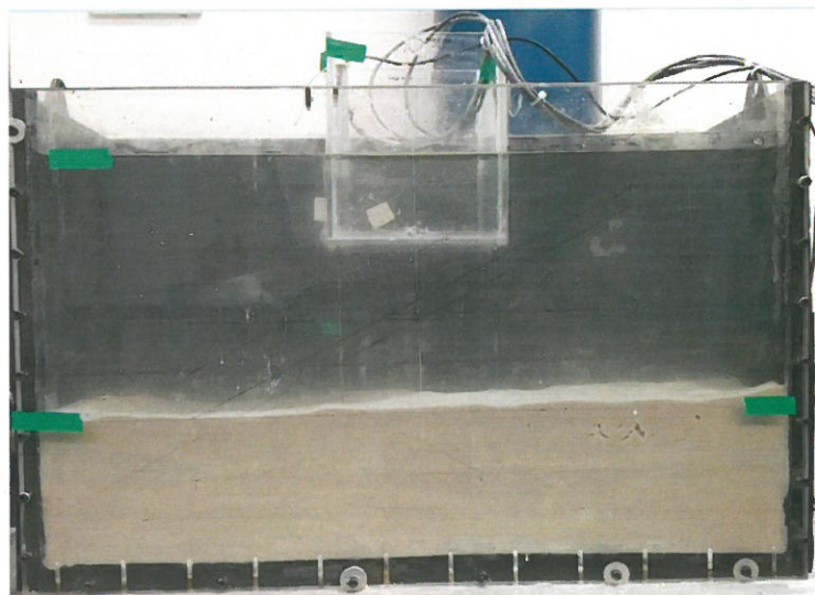
Figure 4.3.1 Experiment 4 setup with 180 mm embedment depth
