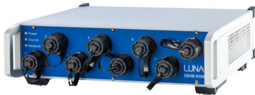
Figure 11: Luna ODiSI 6100 optical distributed sensor interrogator.
