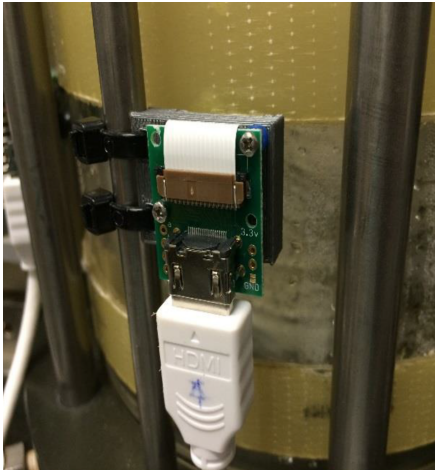
Figure 7: RPi camera set-up using zip ties to mount cameras
