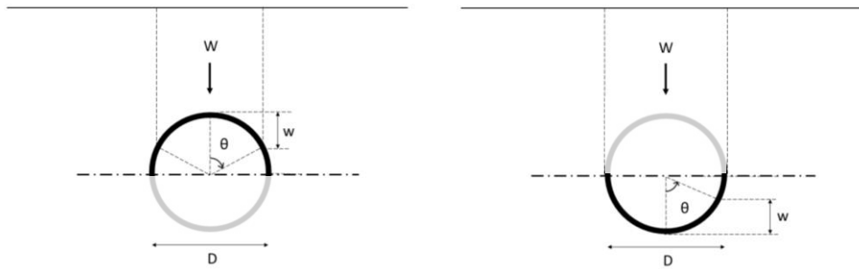
Figure 10. Breakdown of top and bottom half pipes in the analysis
