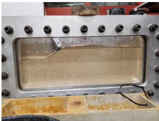
Figure 16(a). Overall setup showing the container tank and the Tekscan handle connected to the sensor during the calibration process.
