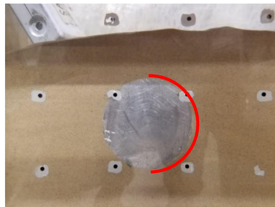
Figure 16(b). A close-up shot of the shallowly buried cylinder, with the red line denoting the position of the I-scan pad wrapped around the cylinder.
