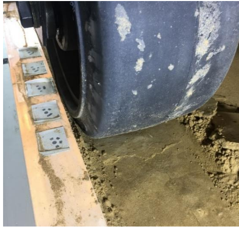
Figure 22 - Upheaval of subgrade in front of wheel in test 2
