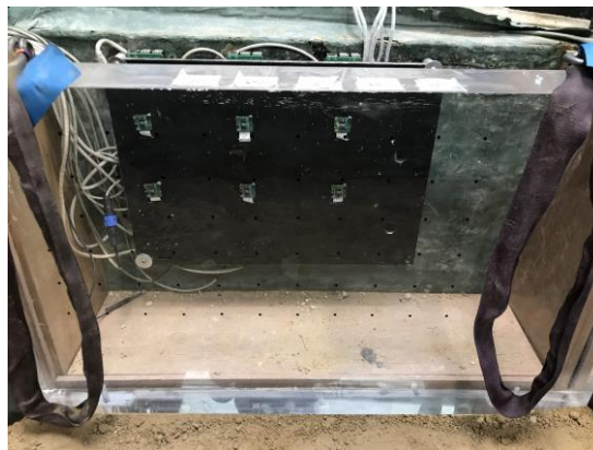
Figure 15 - Camera setup located opposite Perspex window to monitor soil displacement
