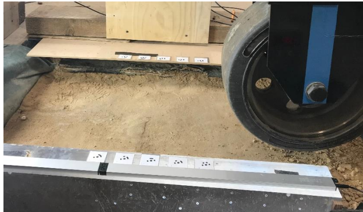
Figure 19 - Layout of control points used in pavement surface reconstruction
