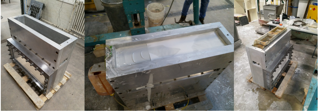
Figure 17: Test box preparation: extension attachment, sand base and greasing (left), clay pouring (centre) and pre-loading (right).
