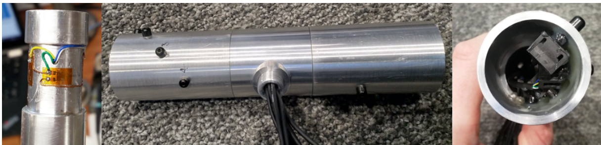
Figure 19: Wiring of the shaft load cell (left), the horizontal bar with sensors and connecting components (centre) and the horizontal bar end view (right).
