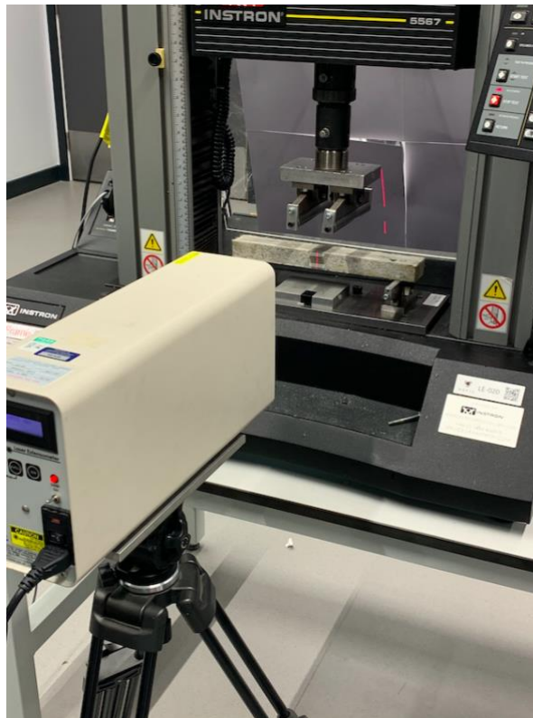
Figure 18 - Experimental set up of flexural 4-point bending testing
