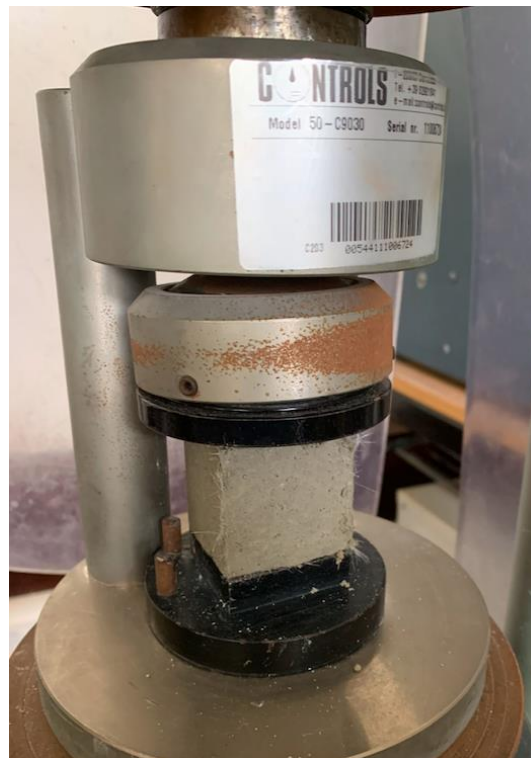
Figure 17 - Uniaxial Compression Testing on Cubic 40×40×40 Specimens
