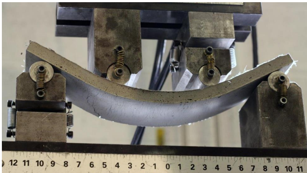
Figure 2 - Ductile Behaviour of ECC or 'Bendable Concrete' (Li & Herbert, 2012)
