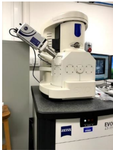
Figure 3.6 ZEISS EVO LS 15 scanning electron microscope (SEM) used for investigating the surface morphology of the specimens
