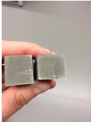
Figure 4.7 Fracture surface of the control sample
